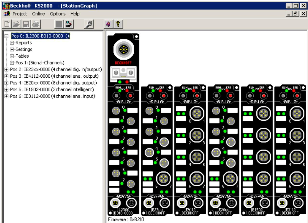
For this test, the fieldbus master (e.g. a PROFIBUS PC Card) should be on the bus and it should transmit data cyclical. Another way to generate cyclic data is, to switch the coupler to *free running* via the KS2000 software.
