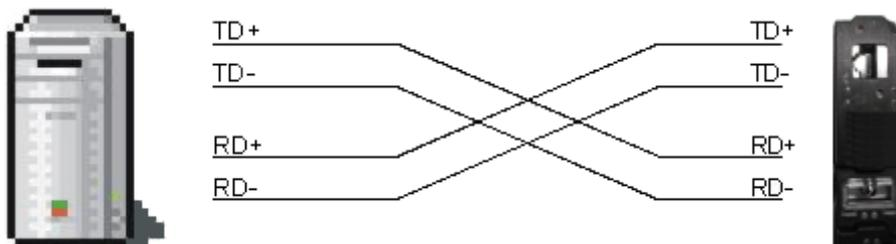
To connect the PC directly to the Fieldbus Box, you must use an Ethernet cable in which the pairs of cores have been crossed (a crossover cable).
