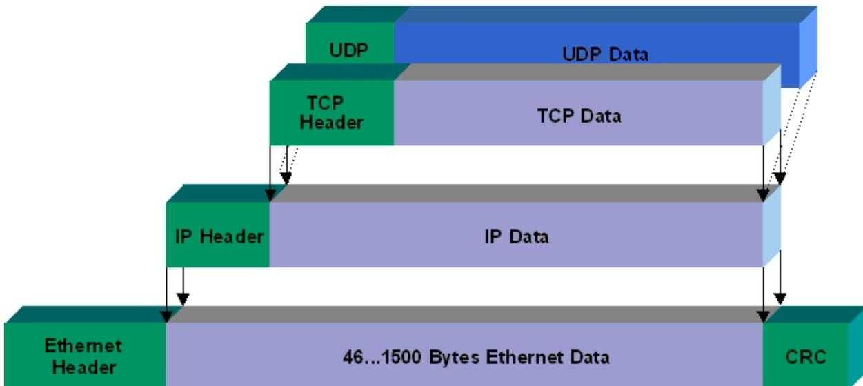
**Protocols running on top of TCP/IP and UDP/IP**
