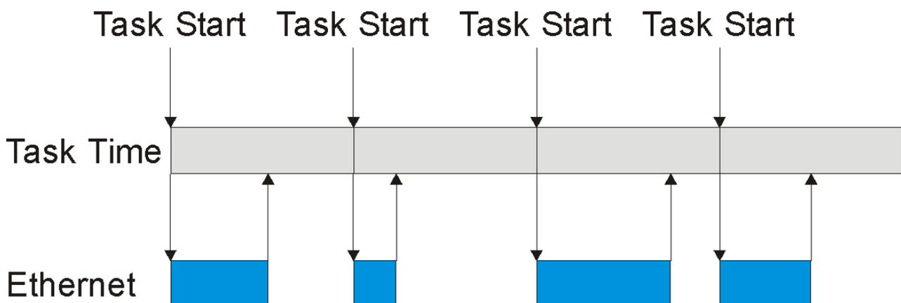
If, after the task time has elapsed, an Ethernet telegram has still not arrived at the PC, only reaching it after the next task has started, then TwinCAT will continue to work with the old input data. In addition, the *MissedCnt* counter is incremented.
