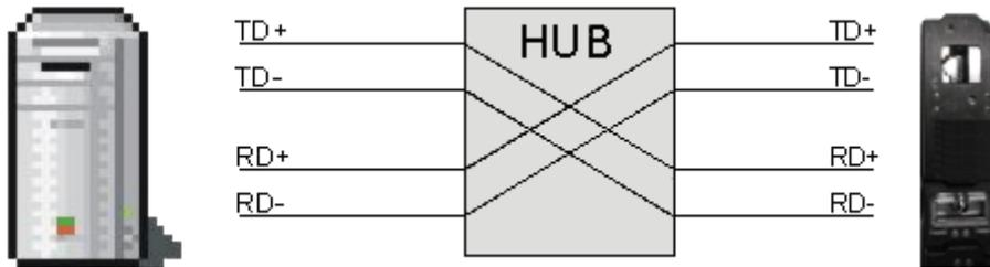
Connect the PC's network card to the hub using a standard Ethernet cable, and connect the hub, again using a standard Ethernet cable, to the Fieldbus Box. Connection via a switch is done in the same way.
