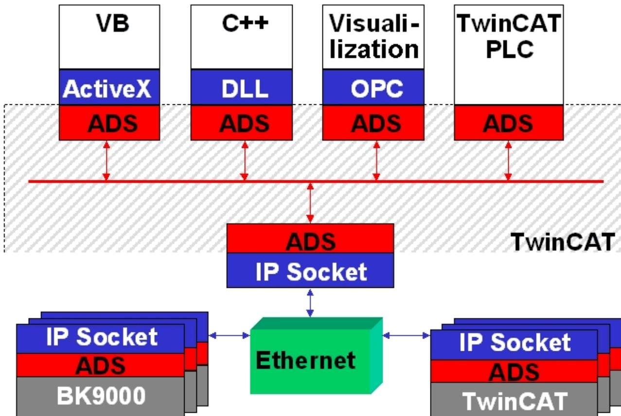
The ADS protocol runs on top of the TCP/IP or UDP/IP protocols. It allows the user within the Beckhoff system to use almost any connecting route to communicate with all the connected devices and to parameterize them. Outside the Beckhoff system a variety of methods are available to exchange data with other software tools.
