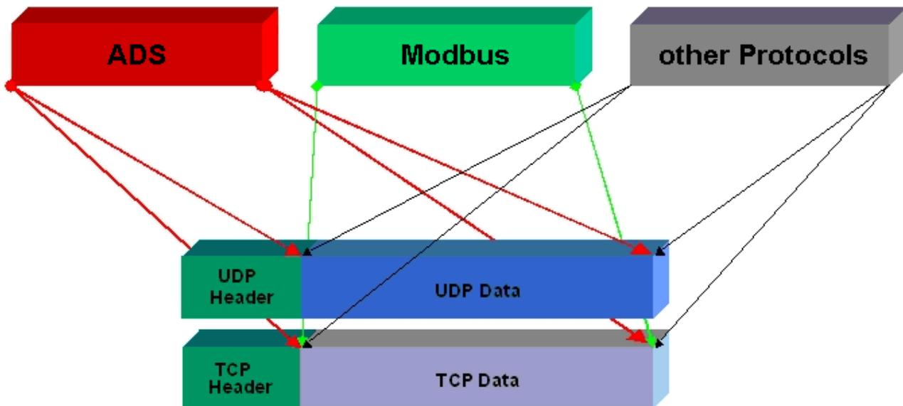
ADS can be used on top of either TCP or UDP, but ModbusTCP is always based on TCP/IP.
