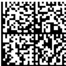
Fig. 4: Example DMC **1P072222SBTNk4p562d71KEL1809 Q1 51S678294**
