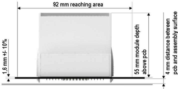
Fig. 15: Mounting distances EJ module - PCB
