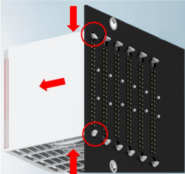
Fig. 26: Disassembly of EJ modules
