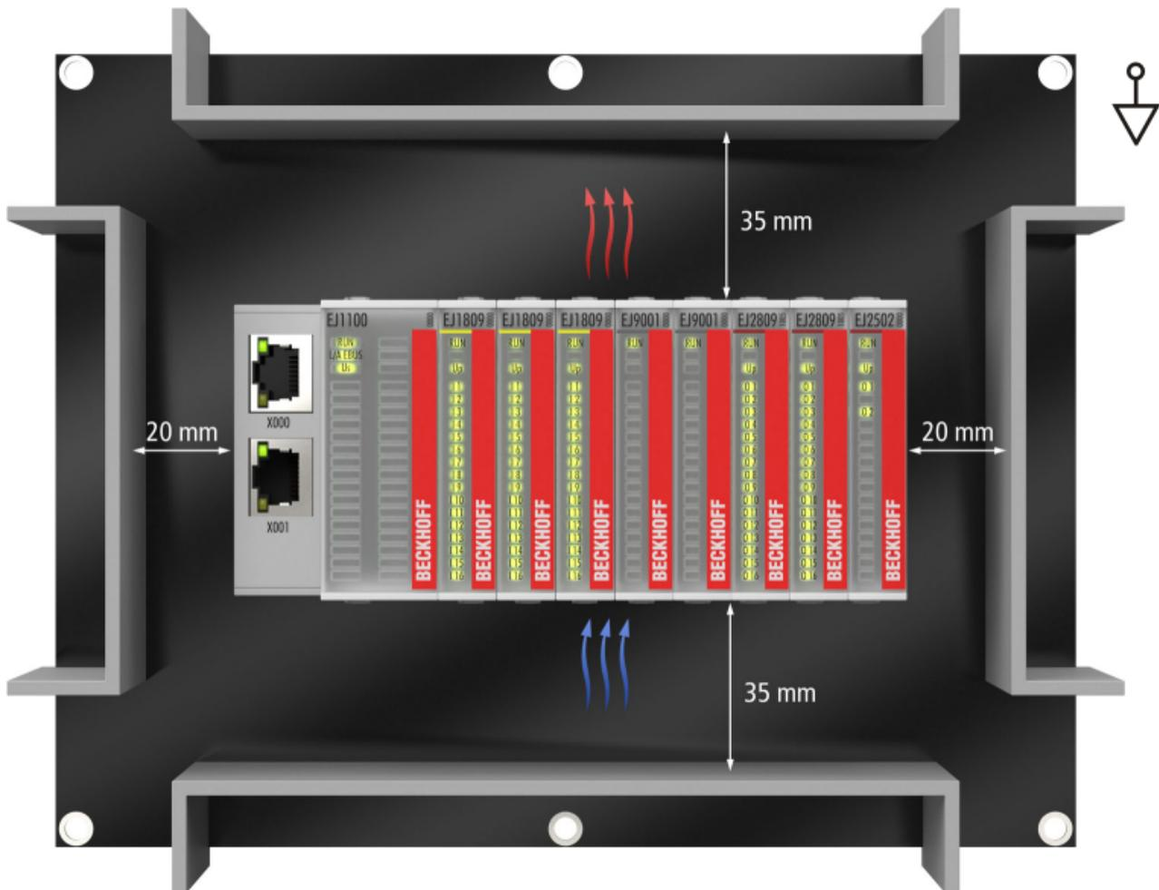
Fig. 16: Recommended distances for standard installation position
