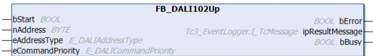
The output value of the DALI control gear is increased over the specified period of 200 ms.
