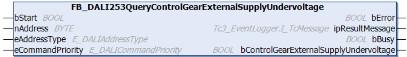
The function block indicates whether an undervoltage has been detected in the external supply voltage of the DALI control gear.
