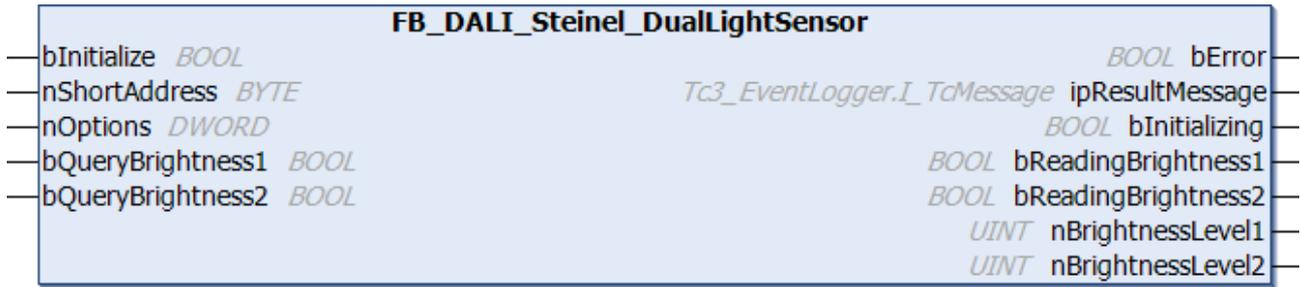
The function block represents the Dual Light Sensor AP/UP DALI sensor from Steinel.
