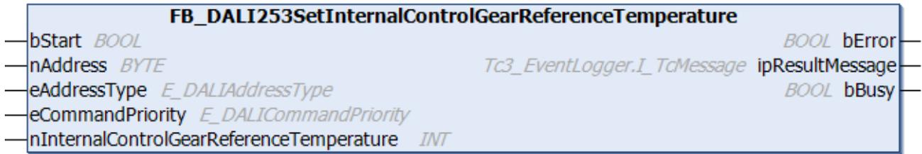
The function block writes the internal reference temperature to the DALI control gear.
