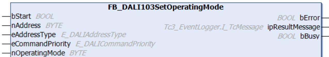
The function block sets the operating mode of the DALI control device (see [operatingMode \[▶ 230\]](#)).
