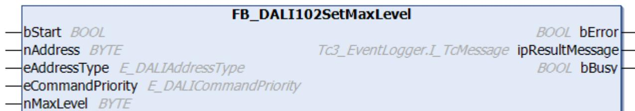
The function block stores the value *nMaxLevel* in the variable [maxLevel \[► 150\]](#) of the DALI control gear.
