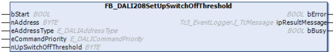
The function block stores the value *nUpSwitchOffThreshold* in the variable [upSwitchOffThreshold](#) [▶ 350] of the DALI control gear.
