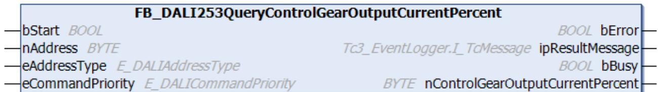
The function block reads the output current as a percentage of the nominal current from the DALI control gear.
