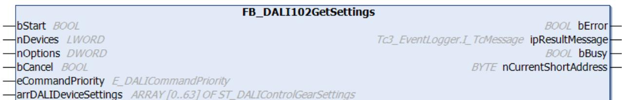
This function block reads several variables (see table [below](#) [▶ 40]) from selected DALI control gears and saves them in the structure [ST\\_DALIControlGearSettings](#) [▶ 852].
