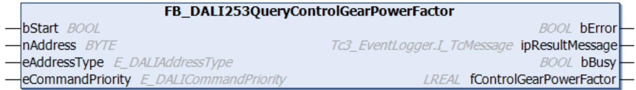
The function block outputs the power factor of the DALI control gear.
