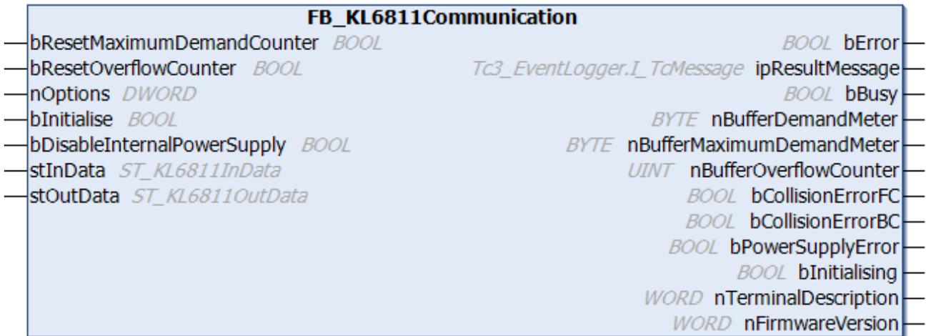
The function blocks for the DALI commands do not directly access the process image of the KL6811, but place the individual DALI commands in a command buffer. The function block FB\_KL6811Communication sequentially reads the DALI commands from the command buffer and forwards them to the KL6811. This prevents multiple function blocks accessing the KL6811 process image at the same time.
