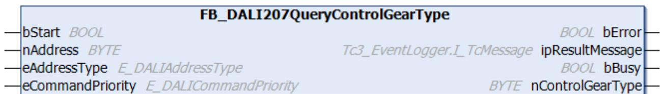
The function block reads the variable `controlGearType` [▶ 330] from the DALI control gear.
