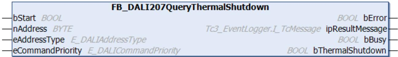
The function block queries whether a thermal shutdown has taken place.
