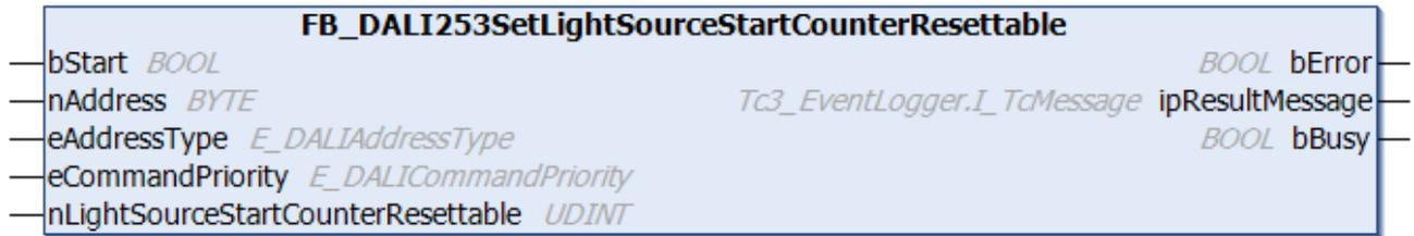
The function block sets the resettable counter for the switching on of the light source to any desired value. The resettable counter is incremented by one each time the light source changes from the Off state to the On state.
