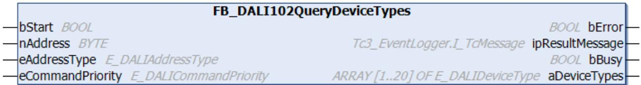
The function block returns a list of all device types supported by the DALI control gear.
