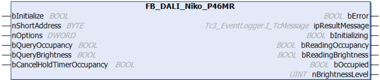
The function block represents the DALI sensors P46MR for surface mounting, P46MR for SnapFit flush mounting and P46MR for flush-mounting box from Niko.
