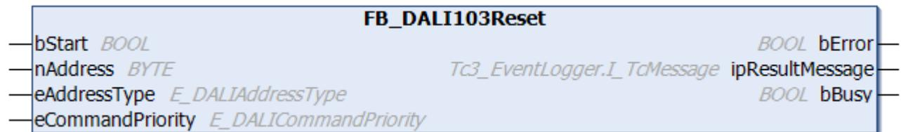
The function block resets all device and instance variables of the DALI control device to their default values (see [resetState \[▶ 231\]](#)).
