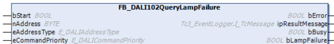
The function block checks whether there is a defect in the lamp of a DALI control gear.
