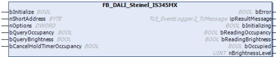
The function block represents the IS 345 MX AP/UP DALI sensor from Steinel.
