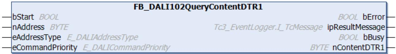
The function block reads the contents of [DTR1 \[► 154\]](#) (Data Transfer Register 1) from the DALI control gear.
