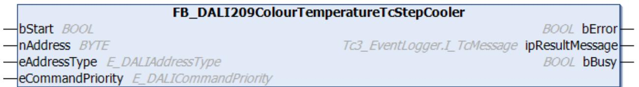
Due to the function block the value [colourTemperatureTc \[▶ 419\]](#) is reduced by 1 Mirek without cross-fading. If the [colourTemperatureTc \[▶ 419\]](#) value already has the same value as [colourTemperatureTcCoolest \[▶ 419\]](#), no change takes place.
