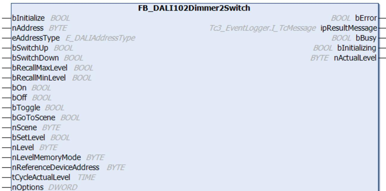
The function block FB\_DALI102Dimmer2Switch provides the main functions for implementing a push-dimmer.
