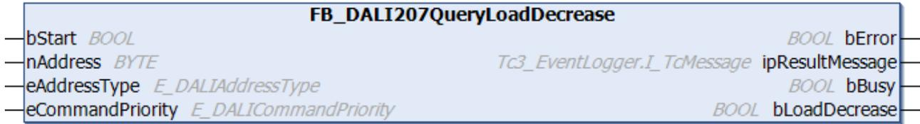
The function block queries whether a significant load decrease (in comparison with the reference power of the system) has been detected.
