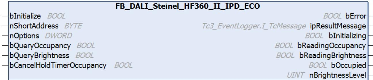
The function block represents the HF 360 II IPD ECO DALI sensor from Steinel.
