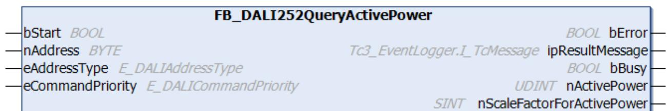
The function block reads the active power from the DALI control gear.
