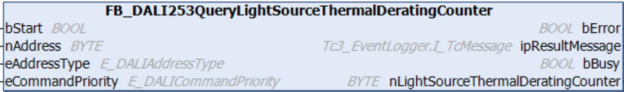
The function block reads the counter that counts the number of times the light source temperature exceeded the limit value.
