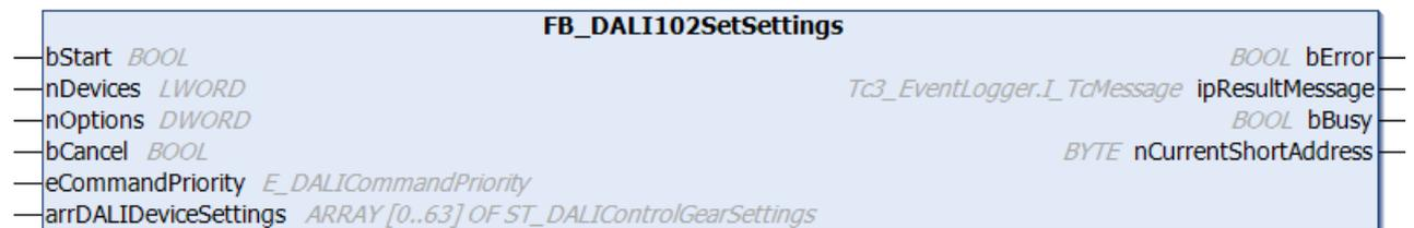
This function block writes the values stored in the structure [ST\\_DALIControlGearSettings](#) [▶ 852] to several variables (see table [below](#) [▶ 40]) of selected DALI control gears in a DALI line.
