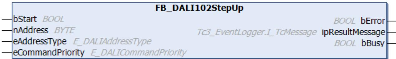
The output value of the DALI control gear is increased by one step.
