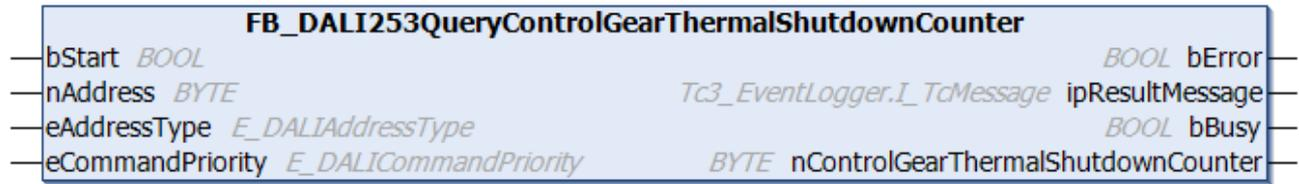
The function block reads the counter of the number of thermal shutdowns of the DALI control gear.
