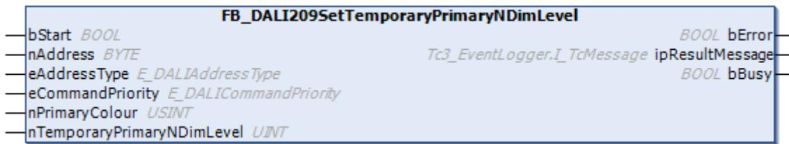
The function block saves the value *nTemporaryPrimaryNDimLevel* in the variable *temporaryPrimaryNDimLevel* [[▶ 419](#)] of the DALI control gear.
