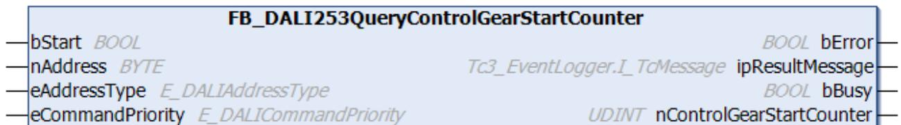
The function block outputs the number of starts of the DALI control gear. The value is incremented after switching on the external power supply.
