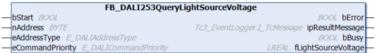
The function block reads the output voltage at the DALI control gear.
