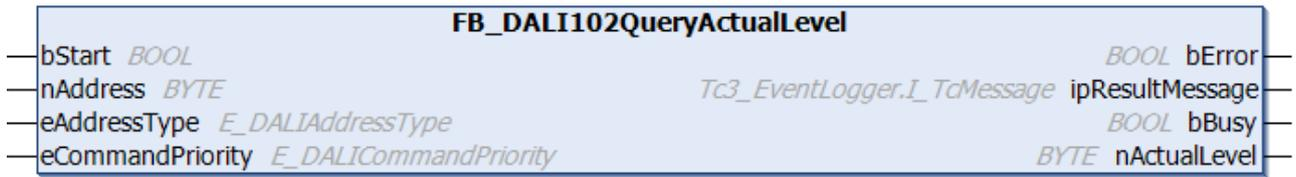
The function block reads the current output value of the DALI control gear (see [actualLevel \[▶ 150\]](#)).
