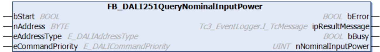
The function block reads the nominal input power of the luminaire from the DALI control gear.
