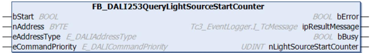
The function block reads the non-resettable counter for the switching on of the light source. The non-resettable counter is incremented by one each time the light source changes from the Off state to the On state. The non-resettable counter cannot be reset or changed.
