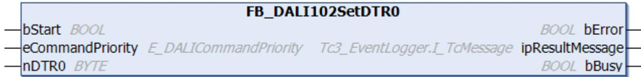
The function block writes to the [DTR0 \[▶ 154\]](#) (Data Transfer Register 0) of all DALI control gears.
