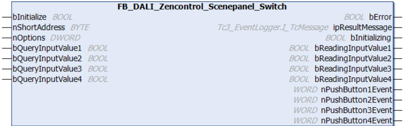
The function block represents the Scenepanel Switch DALI push button interface from Zencontrol.
