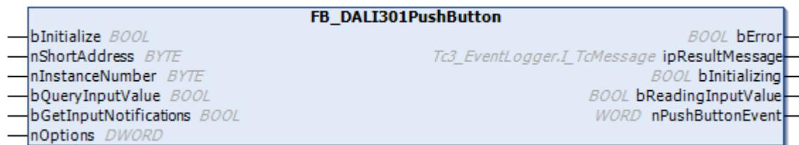
The function block is used for the configuration and operation of an instance of a DALI control device that supports Part 301 (push buttons).
