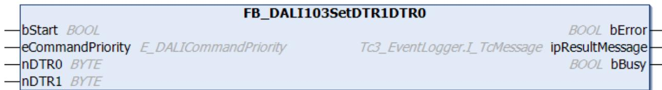
The function block writes the DTR0 (Data Transfer Register 0) and the DTR1 (Data Transfer Register 1) of all DALI control devices.
