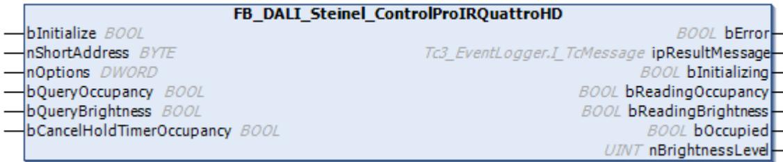
The function block represents the ControlPro IR Quattro HD DALI sensor from Steinel.
