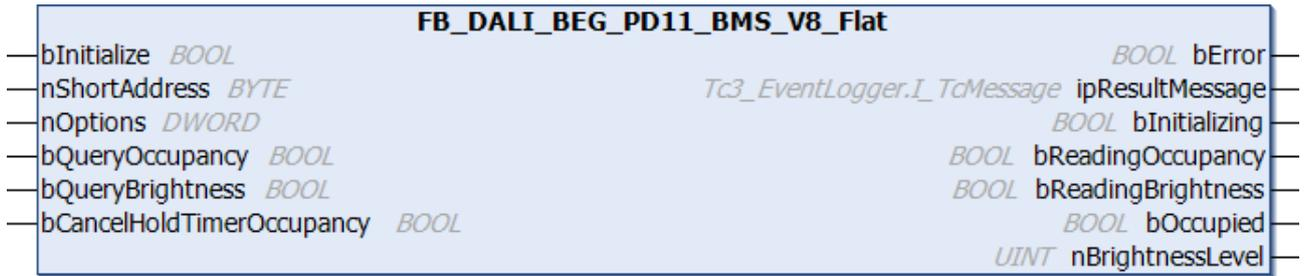
The function block represents the PD11-BMS-FLAT DALI-2 DALI sensor from B.E.G.
