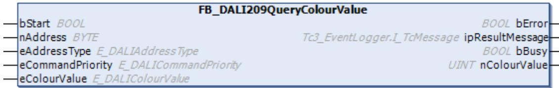
The function block reads the specified variable (color value) from the DALI control gear. The value to be read is defined by *eColourValue*.
