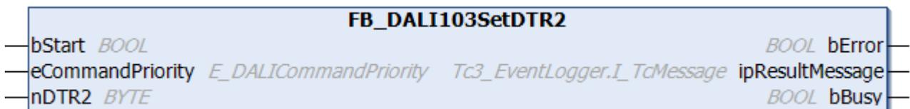
The function block writes to [DTR2 \[▶ 229\]](#) (Data Transfer Register 2) of all DALI control devices.
