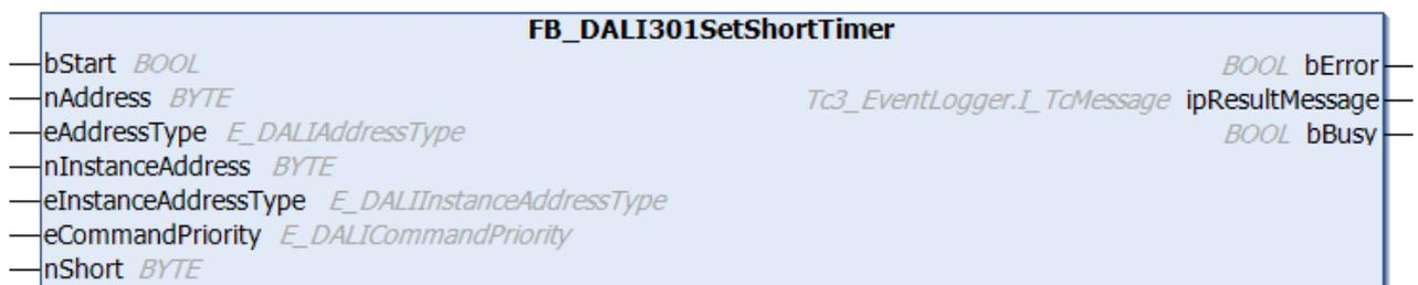
The function block stores the value of *nShort* in the variable *tShort* [▶ 531] of the DALI control device.
