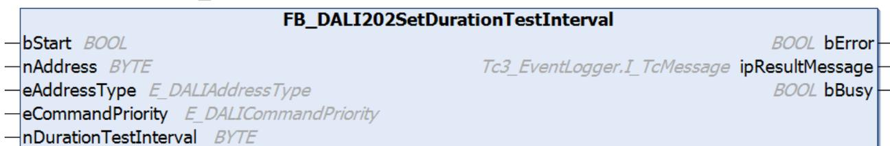
The function block stores the value *nDurationTestInterval* in the variable [durationTestInterval \[▶ 282\]](#) of the DALI control gear.
