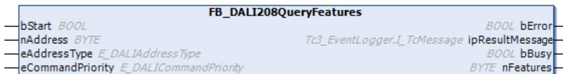
The function block reads the variable [features](#) [▶ 350] from the DALI control gear.
