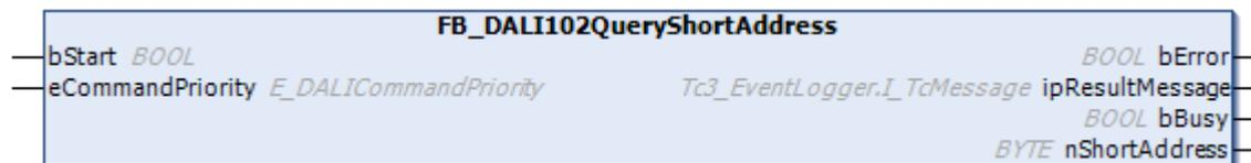
The function block reads the short address ([shortAddress \[▶ 153\]](#)) of the selected DALI control gear.
