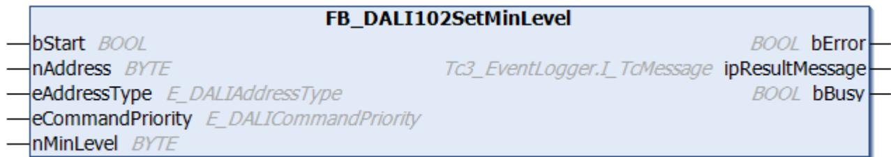
The function block stores the value *nMinLevel* in the variable `minLevel` [[► 150](#)] of the DALI control gear.
