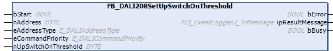
The function block stores the value *nUpSwitchOnThreshold* in the variable *upSwitchOnThreshold* [▶ 350] of the DALI control gear.
