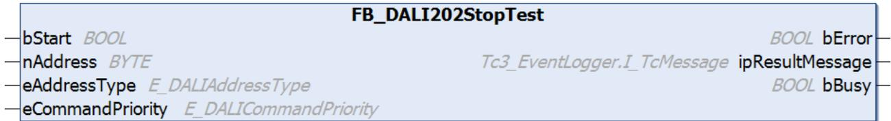
The function block stops a function or duration test.
