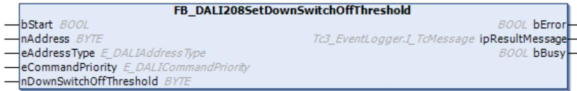
The function block stores the value *nDownSwitchOffThreshold* in the variable *downSwitchOffThreshold* [▶ 350] of the DALI control gear.
