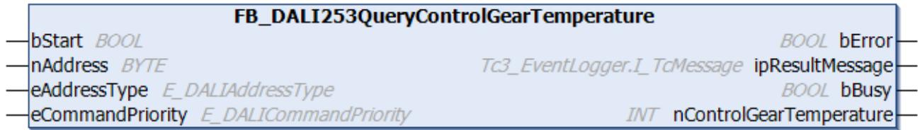
The function block outputs the internal temperature of the DALI control gear.
