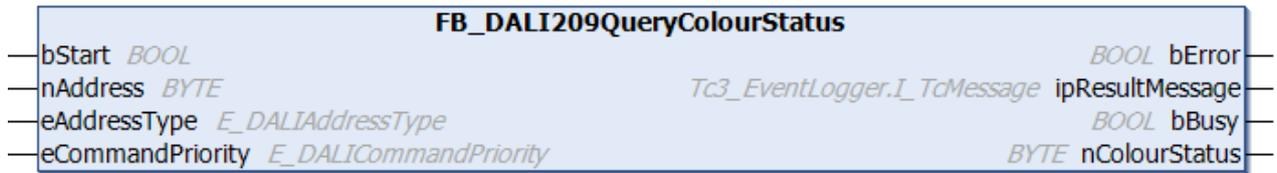
The function block reads the variable `colourStatus` [► 420] from the DALI control gear.
