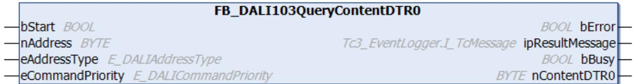
The function block reads the contents of DTR0 [▶ 229] (Data Transfer Register 0) from the DALI control device.
