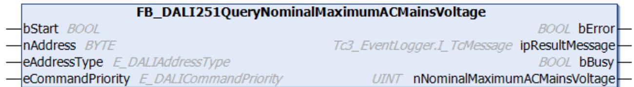
The function block reads the maximum nominal input voltage of the DALI control gear.
