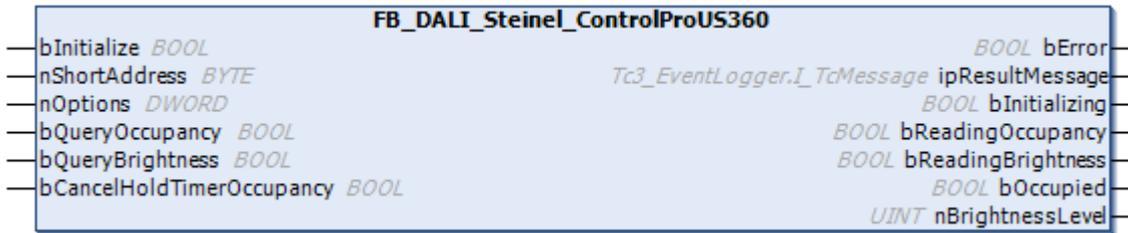
The function block represents the ControlPro US 360 DALI sensor from Steinel.
