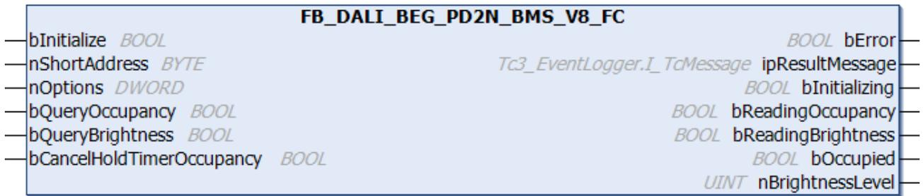
The function block represents the PD2N-BMS-FC DALI-2 DALI sensor from B.E.G..
