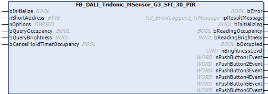
The function block represents the MSensor G3 SFI 30 PIR 5DPI, MSensor G3 SFI 30 PIR 10DPI or MSensor G3 SFI 30 PIR 16DPI DALI sensor from Tridonic.
