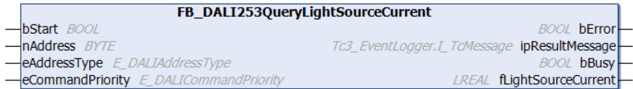
The function block reads the current consumption of the light source.
