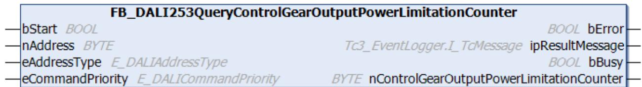
The function block reads the counter of the number of exceedances of the output power limit value at the DALI control gear.
