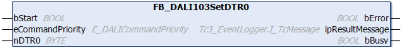
The function block writes to the [DTR0 \[► 229\]](#) (Data Transfer Register 0) of all DALI control devices.
