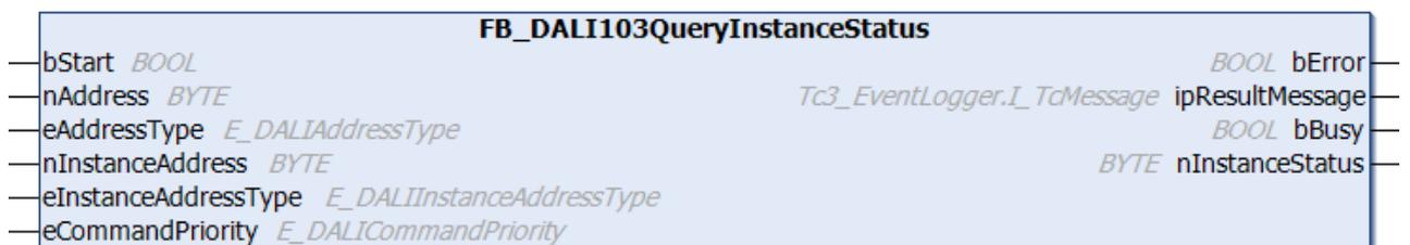
The function block reads the status of the selected instance from the DALI control device.
