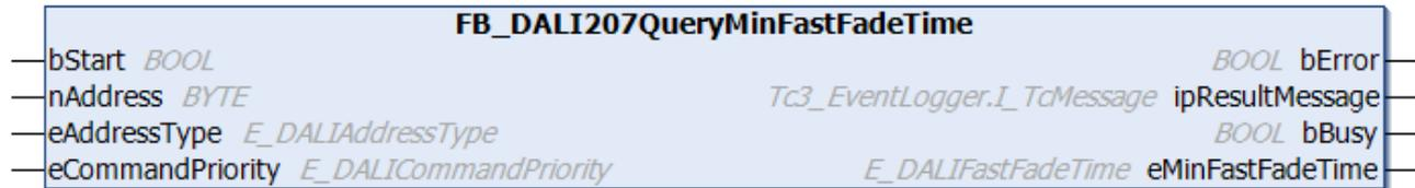
The function block reads the variable `minFastFadeTime` [▶ 329] from the DALI control gear.
