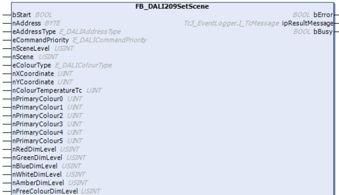
The function block can be used to assign a specific lighting value to a scene.
