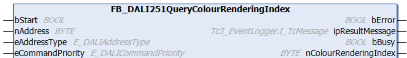
The function block reads the color rendering index from the DALI control gear.
