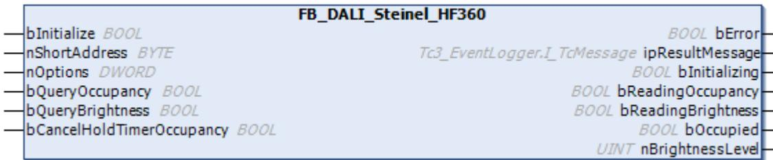
The function block represents the HF 360 DALI sensor from Steinel.
