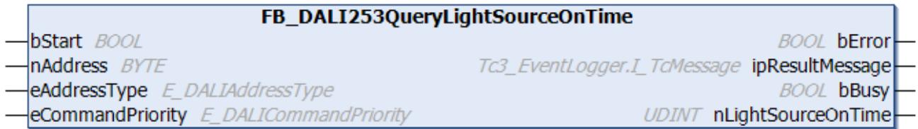
The function block reads the non-resettable operating hour counter of the light source. If the light source is switched on, the non-resettable operating hour counter is incremented by one every second.
