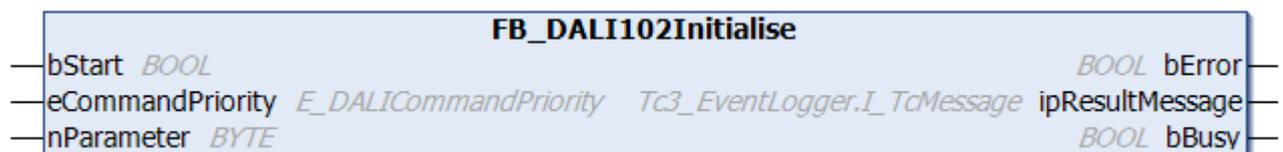
The function block prepares the addressing of the DALI control gears.
