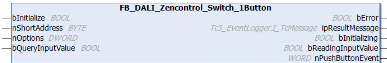
The function block represents the Switch 1 Button DALI push button interface from Zencontrol.
