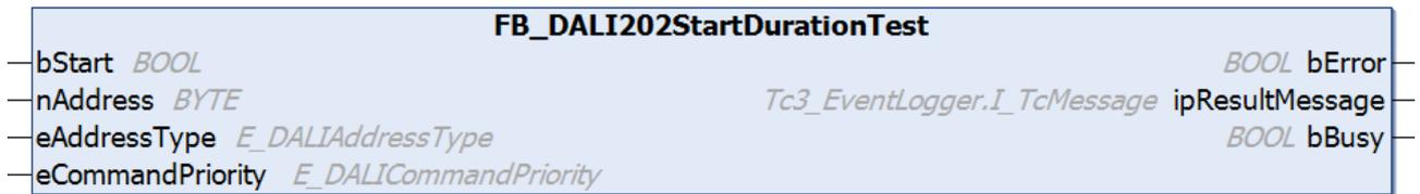
The function block starts a duration test.
