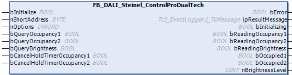
The function block represents the ControlPro Dual Tech US Dali sensor from Steinel.
