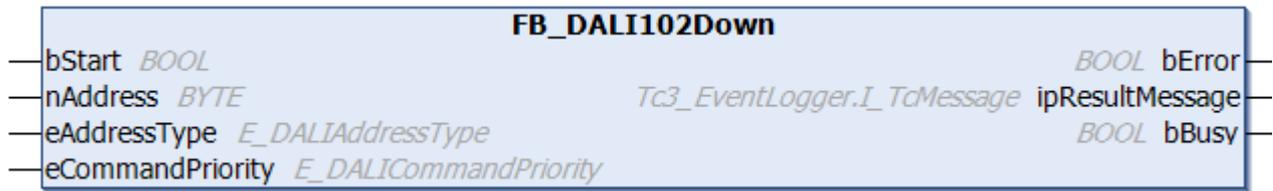
The output value of the DALI control gear is reduced over the specified period of 200 ms.
