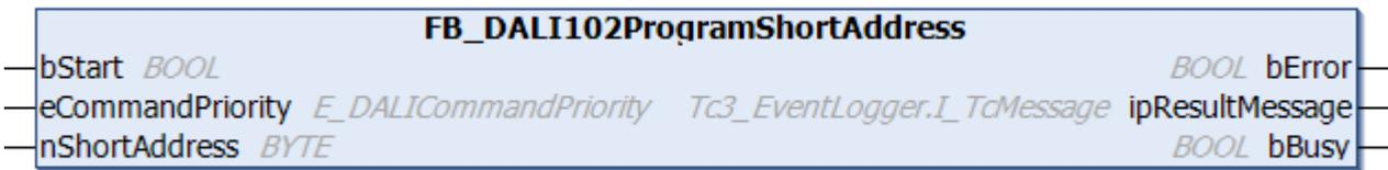
The function block stores the value *nShortAddress* as a short address in the variable *shortAddress* [[▶ 153](#)] for all selected DALI control gears.
