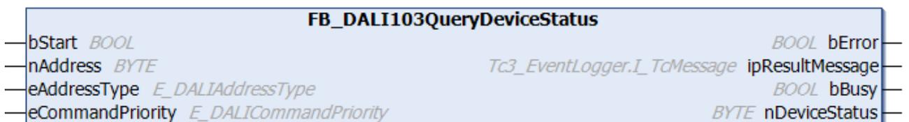
The function block reads the status of the DALI control device.
