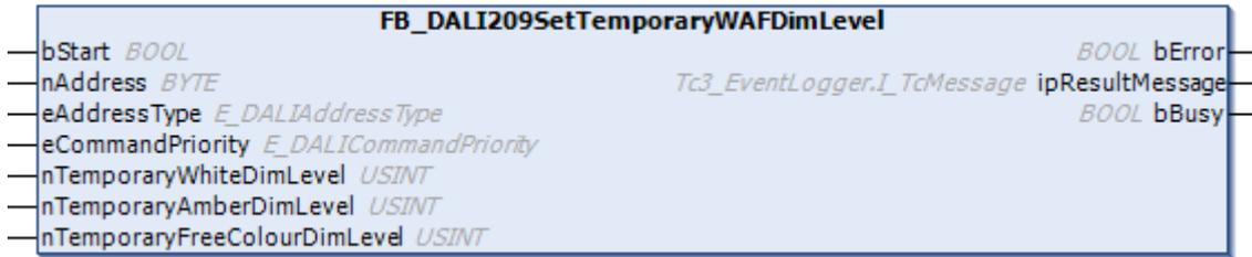
The function block saves the values *nTemporaryWhiteDimLevel*, *nTemporaryAmberDimLevel* and *nTemporaryFreeColourDimLevel* in the variables [temporaryWhiteDimLevel \[▶ 419\]](#), [temporaryAmberDimLevel \[▶ 419\]](#) and [temporaryFreeColourDimLevel \[▶ 419\]](#) of the DALI control gear.
