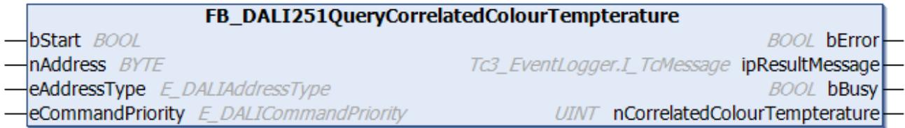
The function block reads the correlated color temperature from the DALI control gear.
