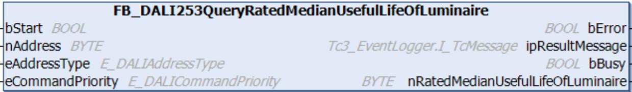
The function block indicates the estimated average lifetime of the complete luminaire, including all individual components.
