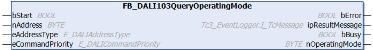
The function block reads the variable `operatingMode` [► 230] from the DALI control device.
