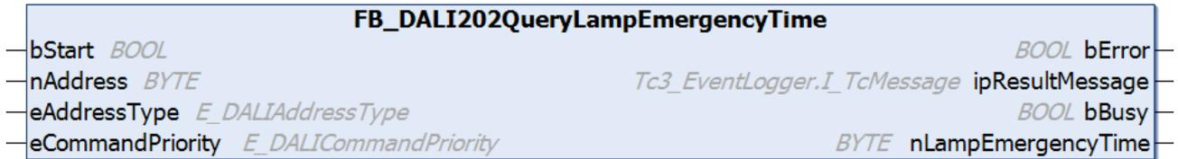
The function block reads the variable `lampEmergencyTime` [▶ 282] from the DALI control gear.
