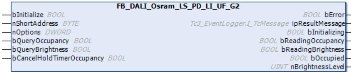
The function block represents the LS/PD LI UF G2 DALI sensor from Osram.
