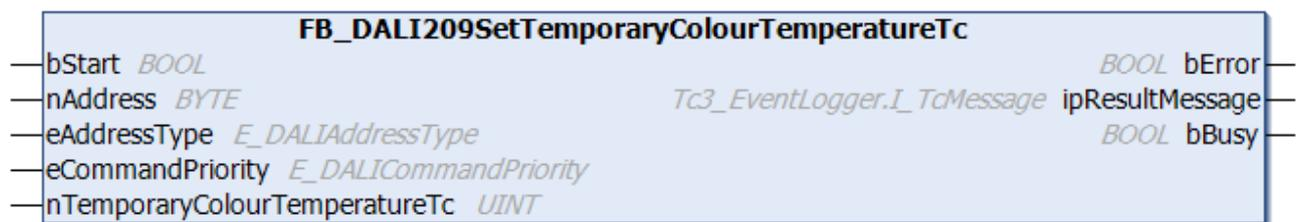
The function block saves the value *nTemporaryColourTemperatureTc* in the variable [temporaryTemperatureTc](#) [▶ 419] of the DALI control gear.
