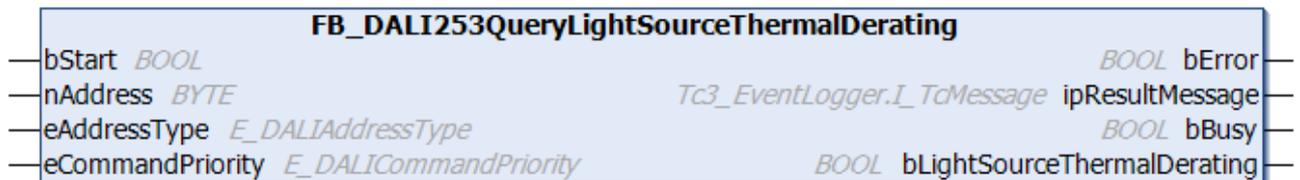
The function block indicates whether the light source temperature is higher than the specified limit value.
