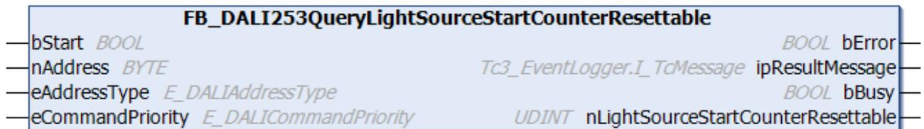
The function block reads the resettable counter for the switching on of the light source. The resettable counter is incremented by one each time the light source changes from the Off state to the On state.
