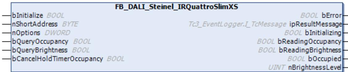
The function block represents the IR Quattro Slim XS DALI sensor from Steinel.
