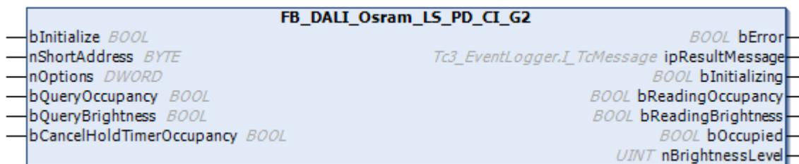
The function block represents the LS/PD CI G2 DALI sensor from Osram.
