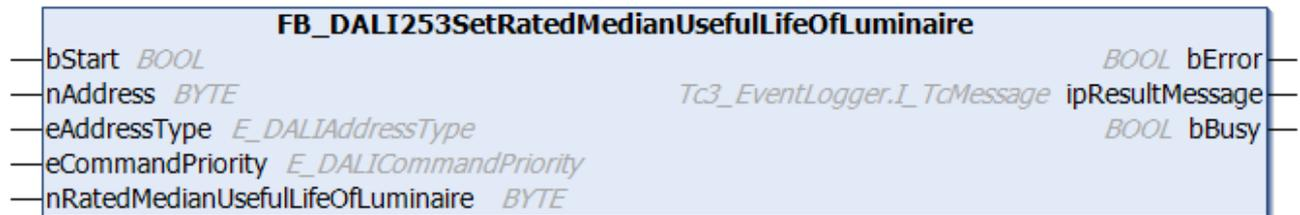
The function block writes the estimated average lifetime of the complete luminaire to the DALI control gear.
