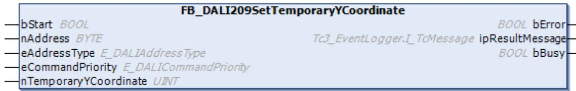
The function block saves the value *nTemporaryYCoordinate* in the variable `temporaryYCoordinate` [▶ 419] of the DALI control gear.
