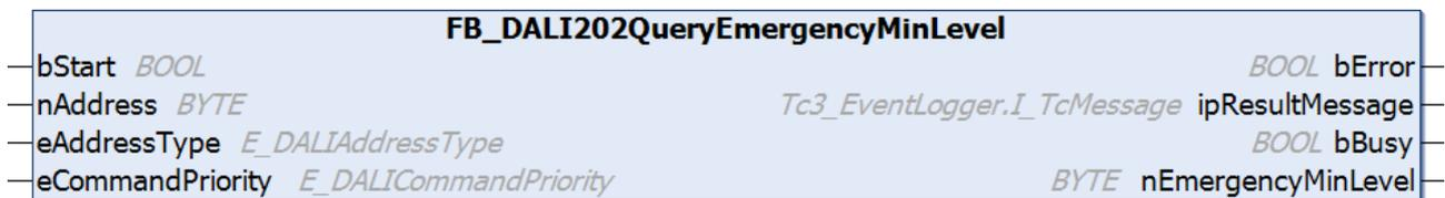
The function block reads the variable [emergencyMinLevel \[▶ 281\]](#) from the DALI control gear.
