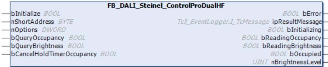
The function block represents the ControlPro Dual HF DALI sensor from Steinel.
