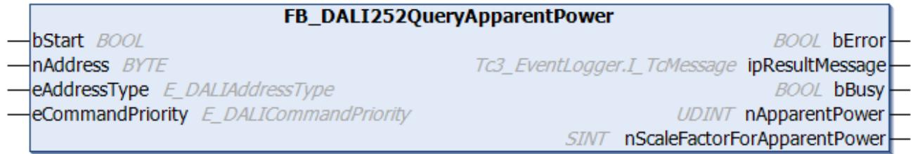
The function block reads the apparent power from the DALI control gear.
