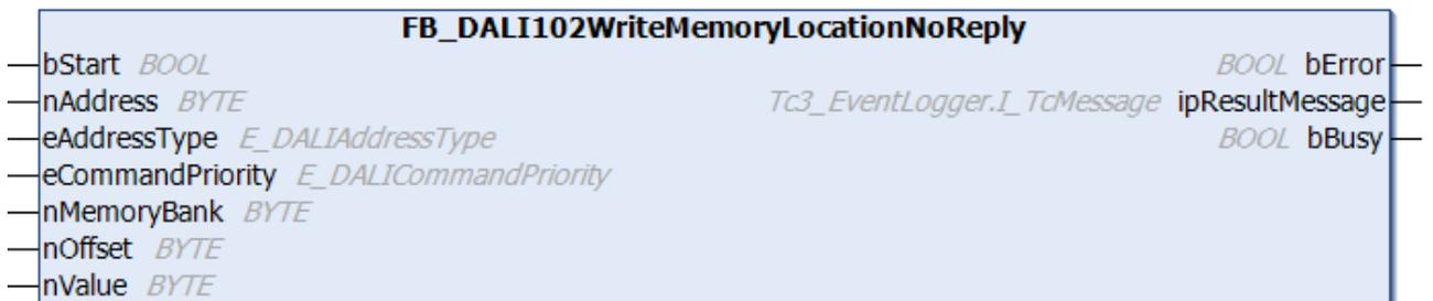
The value *nValue* is written in the memory bank of the DALI control gear. The corresponding memory bank is specified by the input variable *nMemoryBank*, the address within the memory bank by the input variable *nOffset*.
