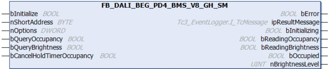
The function block represents the PD4-BMS-GH-SM DALI-2 DALI sensor from B.E.G..
