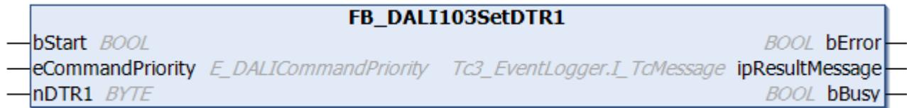
The function block writes to [DTR1 \[► 229\]](#) (Data Transfer Register 1) of all DALI control devices.
