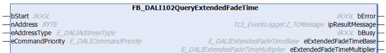
This function block reads the variables [extendedFadeTimeBase](#) [▶ 152] and [extendedFadeTimeMultiplier](#) [▶ 152] from the DALI control gear. The Extended Fade Time (100 ms to 16 min) can be calculated from the product of the two variables.
