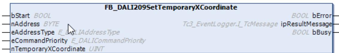
The function block saves the value *nTemporaryXCoordinate* in the variable [temporaryXCoordinate \[▶ 418\]](#) of the DALI control gear.
