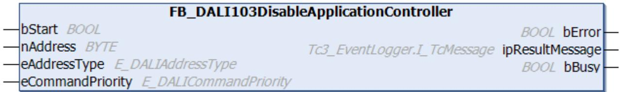
The function block deactivates the application controller (see [applicationActive](#) [▶ 230]).
