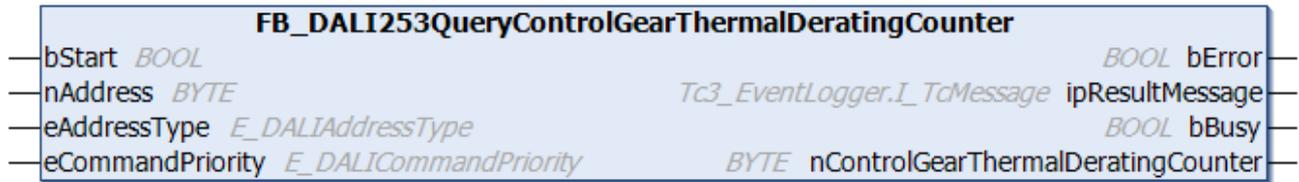
The function block reads the counter that counts the number of times the temperature limit value inside the DALI control gear is exceeded.
