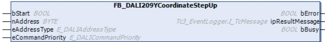
The function block increases the variable `yCoordinate` [▶ 419] by 256 steps (256 / 65536) without cross-fading.
