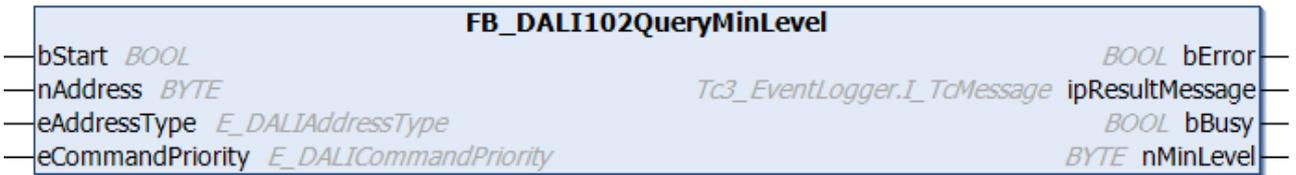
The function block reads the variable `minLevel` [► 150] from the DALI control gear.
