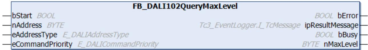
The function block reads the variable `maxLevel` [▶ 150] from the DALI control gear.
