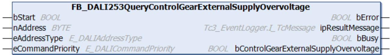
The function block indicates whether an overvoltage has been detected in the external supply voltage of the DALI control gear.
