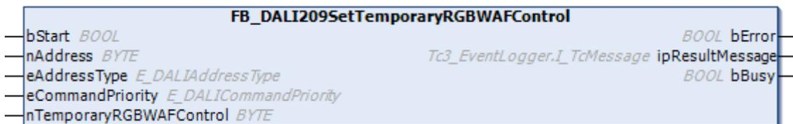
The function block saves the value *nTemporaryRGBWAFControl* in the variable [temporaryRGBWAFControl](#) [▶ 420] of the DALI control gear.
