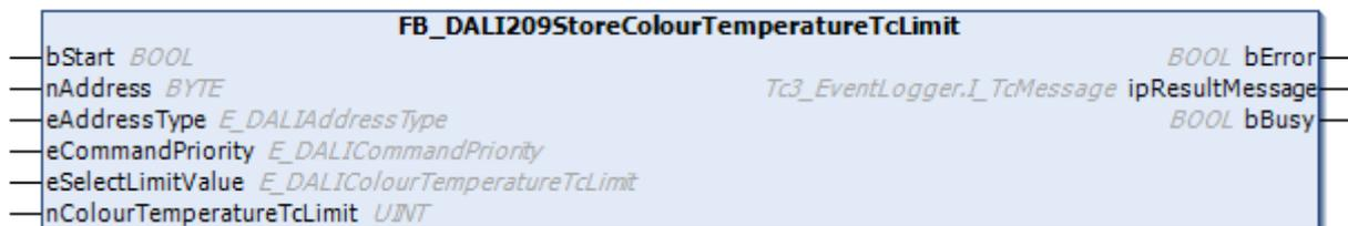
Depending on the specification of *eSelectLimitValue*, the function block saves the value *nColourTemperatureTcLimit* in the variables *colourTemperatureTcCoolest*, *colourTemperatureTcWarmest*, *colourTemperatureTcPhysicalCoolest* or *colourTemperatureTcPhysicalWarmest* of the DALI control gear.
