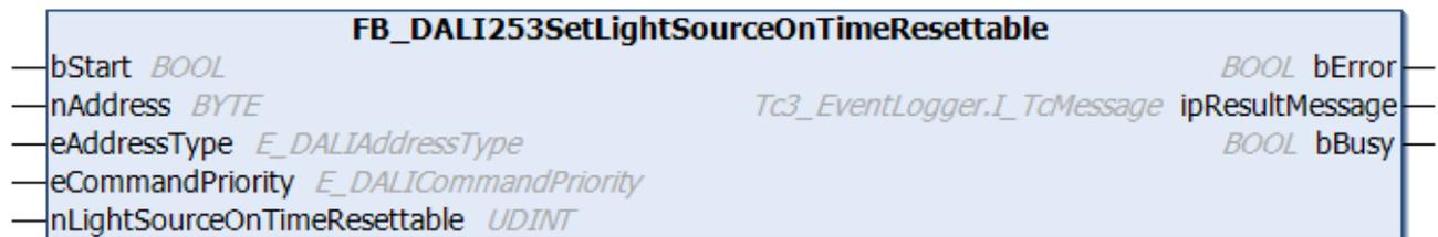
The function block sets the resettable operating hour counter of the light source to any desired value. If the light source is switched on, the resettable operating hour counter is incremented by one every second.
