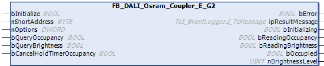
The function block represents the DALI COUPLER E G2 DALI sensor from Osram.
