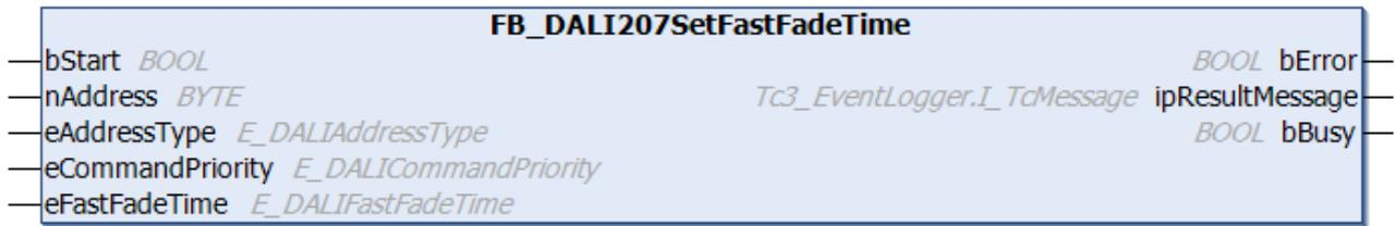
The function block saves the value *eFastFadeTime* in the variable *fastFadeTime* [▶ 330] of the DALI control gear.
