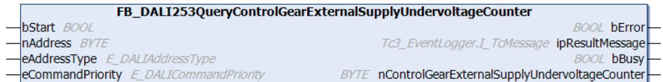
The function block reads the counter for the detected undervoltage events of the external supply voltage of the DALI control gear.
