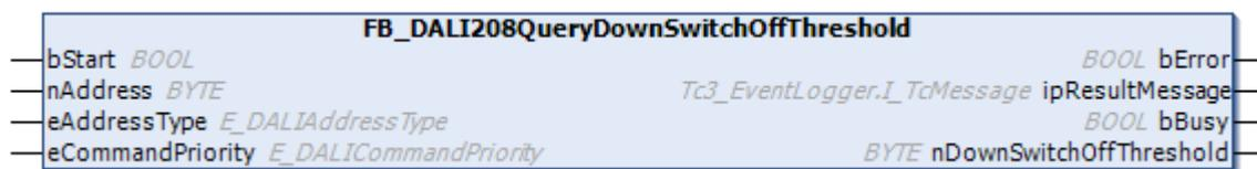
The function block reads the variable [downSwitchOffThreshold](#) [▶ 350] from the DALI control gear.
