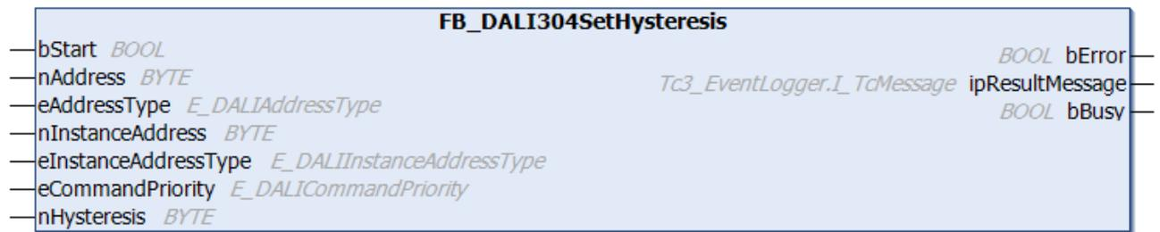
The function block stores the value *nHysteresis* in the variable [hysteresis](#) [[▶ 578](#)] of the DALI control device. The value is stated in %. The permissible value range is between 0% and 25%.
