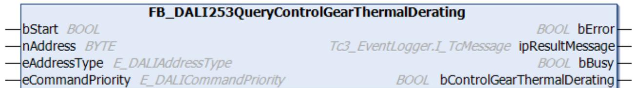
The function block indicates whether the internal temperature is higher than the specified limit value in the DALI control gear.
