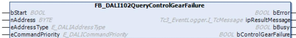
The function block checks whether there is a defect in one or more DALI control gears.
