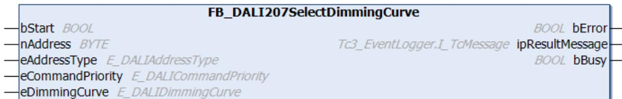
The function block saves the value *eDimmingCurve* in the variable [dimmingCurve](#) [▶ 331] of the DALI control gear.
