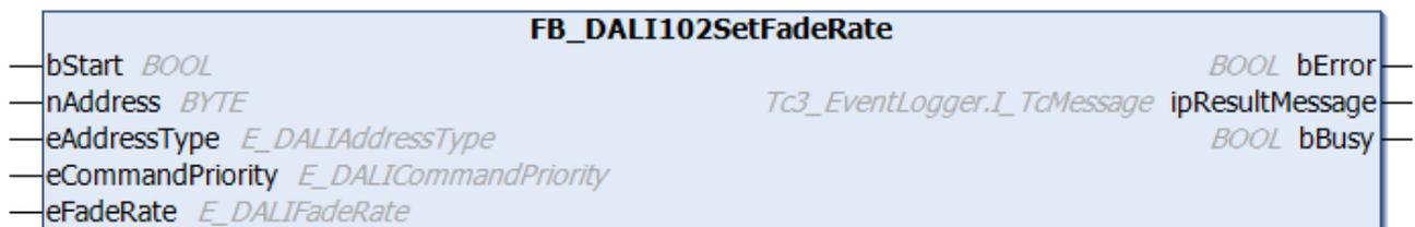
The function block sets the [fadeRate \[▶ 150\]](#) to the value *eFadeRate*.
