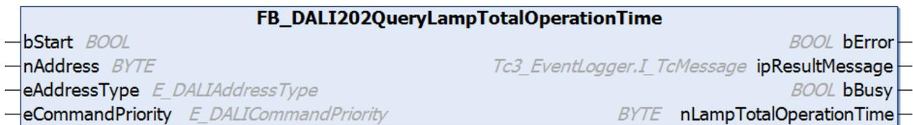
The function block reads the variable [lampTotalOperationTime \[▶ 283\]](#) from the DALI control gear.
