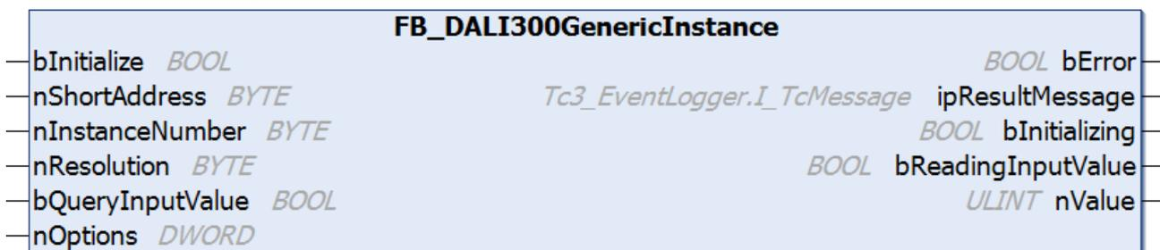
The function block is used for the direct reading of generic values of an instance of a DALI control device that supports Part 103 (instance type 0).
