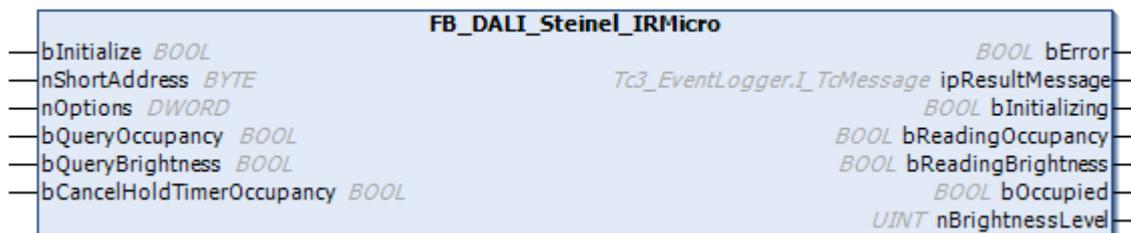
The function block represents the IR Micro DALI sensor from Steinel.
