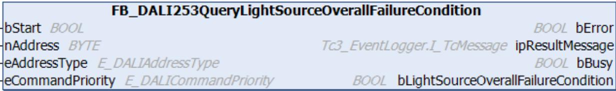
The function block outputs the status of `lampFailure` [▶ 153] at the DALI control gear.
