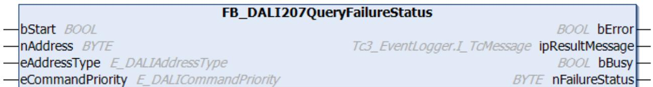
The function block reads the failure status from the DALI control gear (see [failureStatus](#) [▶ 330]).
