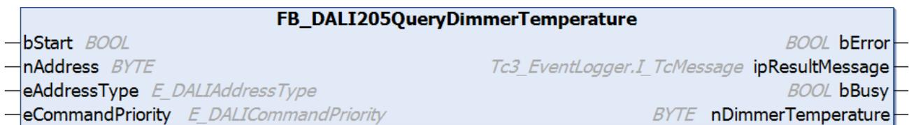
The function block reads the current operating temperature from the DALI control gear (see [dimmerTemperature \[▶ 305\]](#)).
