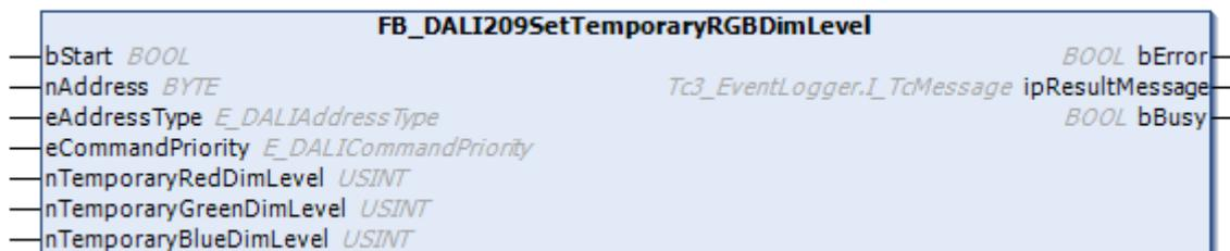
The function block saves the values `nTemporaryRedDimLevel`, `nTemporaryGreenDimLevel` and `nTemporaryBlueDimLevel` in the variables `temporaryRedDimLevel` [▶ 419], `temporaryGreenDimLevel` [▶ 419] and `temporaryBlueDimLevel` [▶ 419] of the DALI control gear.
