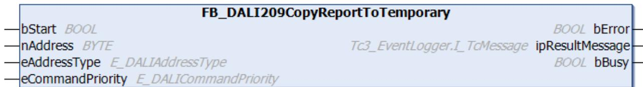
The function block copies the contents of the variables with the color settings to the variables for the temporary color settings.
