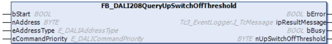
The function block reads the variable `upSwitchOffThreshold` [► 350] from the DALI control gear.
