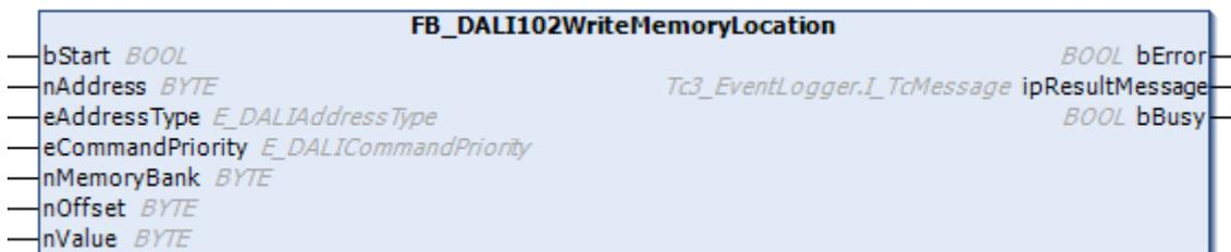
The value *nValue* is written in the memory bank of the DALI control gear. The corresponding memory bank is specified by the input variable *nMemoryBank*, the address within the memory bank by the input variable *nOffset*.
