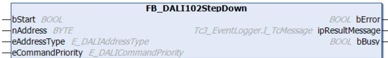
The output value of the DALI control gear is reduced by one step.
