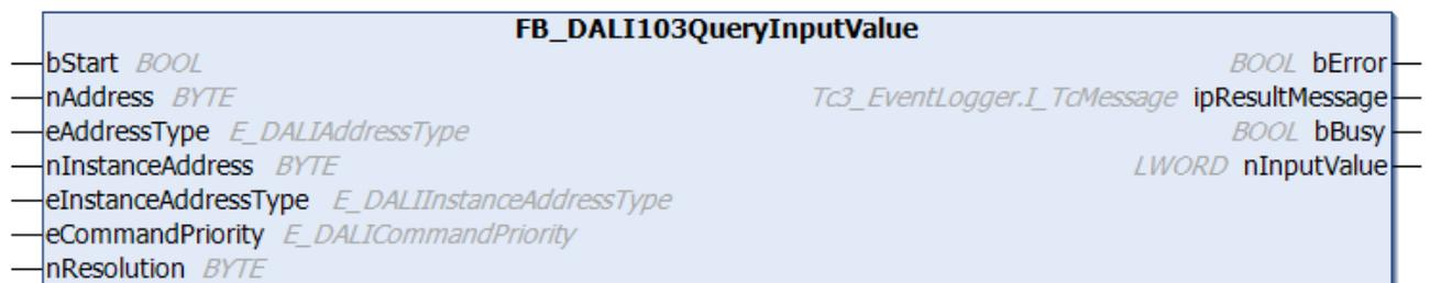
The function block queries the input value (see [inputValue](#) [▶ 232]) of the selected instance of the DALI control device.
