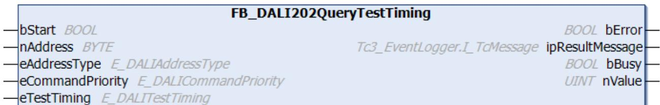
Depending on the input *eTestTiming*, this function block reads out the settings for the function and duration test from the DALI control gear.
