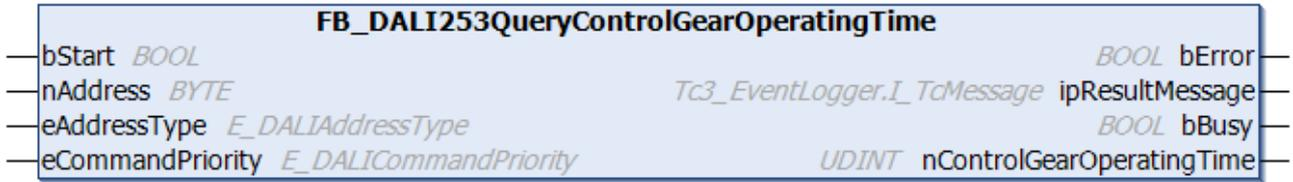
The function block reads the operating time of the DALI control gear.
