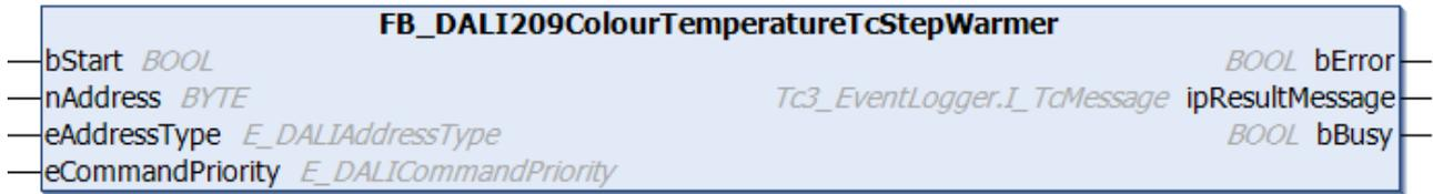
Due to the function block the value `colourTemperatureTc` [▶ 419] is increased by 1 Mirek without cross-fading. If the `colourTemperatureTc` [▶ 419] value already has the same value as `colourTemperatureTcWarmest` [▶ 419], no change takes place.
