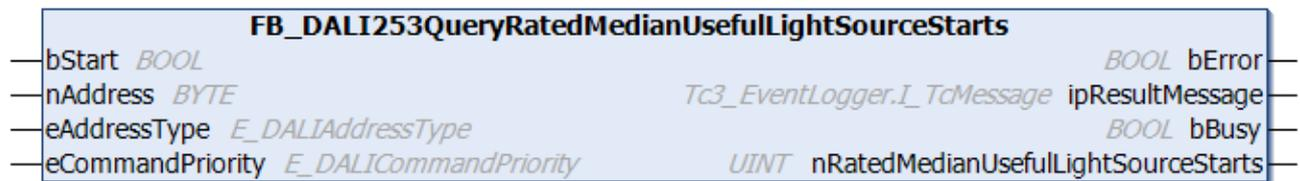
The function block indicates the average number of possible starts of the complete luminaire, including all individual components.
