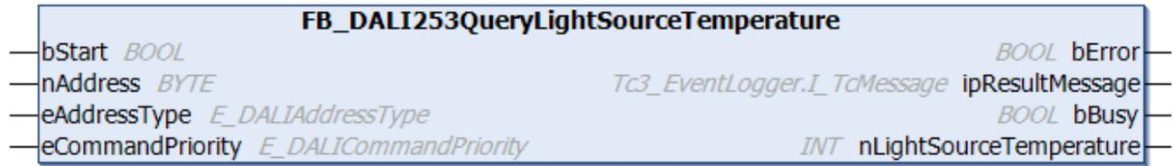
The function block indicates the temperature of the light source.
