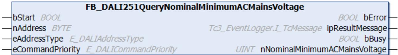
The function block reads the minimum nominal input voltage of the DALI control gear.
