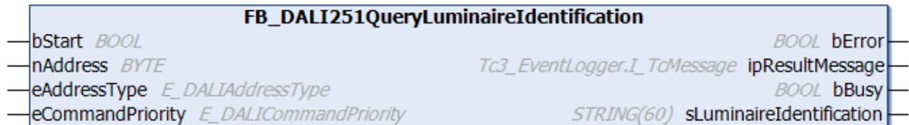
The function block reads the identification designation of the luminaire from the DALI control gear.
