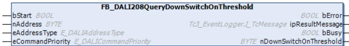
The function block reads the variable `downSwitchOnThreshold` [► 350] from the DALI control gear.
