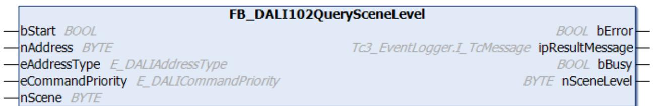
The function block reads the output value from the DALI control gear for the specified scene *nScene*.
