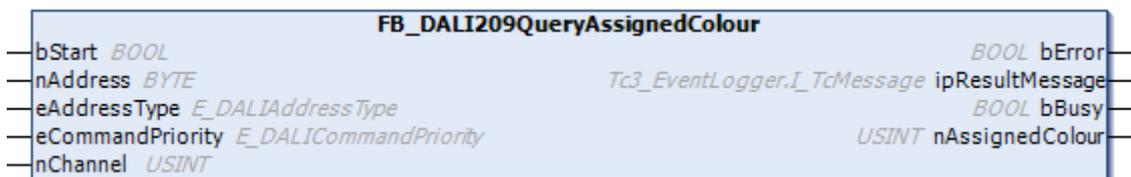
The function block reads the variable [assignedColour](#) [▶ 419] from the DALI control gear.
