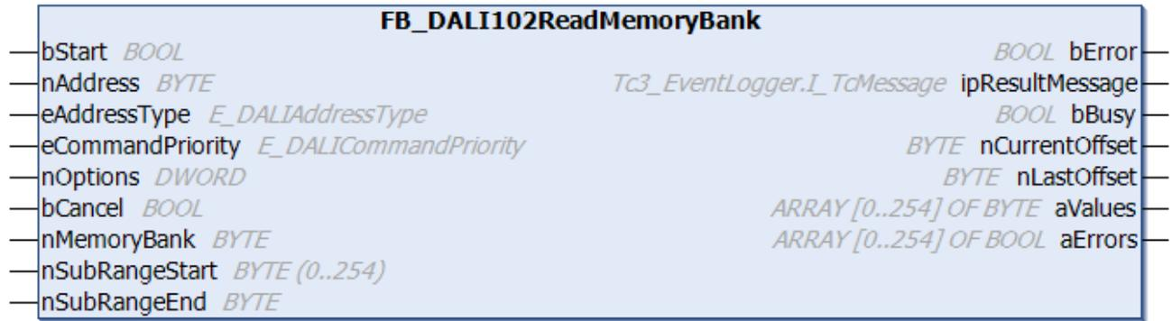
The specified memory bank of the DALI control gear is read (see [Memory banks](#) [▶ 16]). The memory bank is specified by the parameter *nMemoryBank*. The range to be read can be limited with the help of the parameters *nSubRangeStart* and *nSubRangeEnd*.
