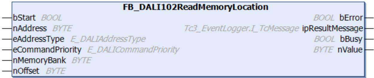
One byte is read from the memory bank of the DALI control gear. The memory bank is specified by the parameter *nMemoryBank* and the address within the memory bank by the parameter *nOffset*.
