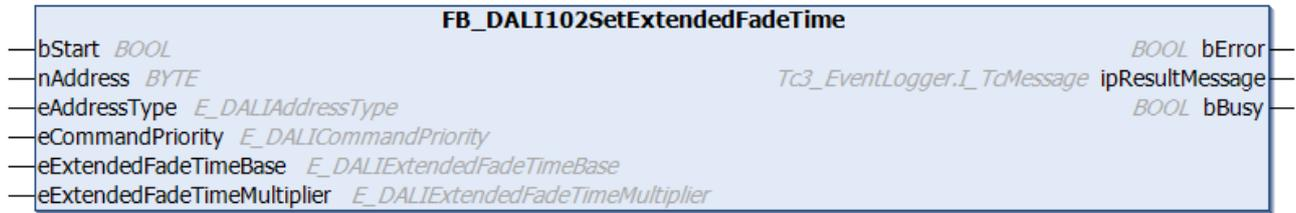
This function block writes the values *eExtendedFadeTimeBase* and *eExtendedFadeTimeMultiplier* to the variables [extendedFadeTimeBase \[▶ 152\]](#) and [extendedFadeTimeMultiplier \[▶ 152\]](#).
