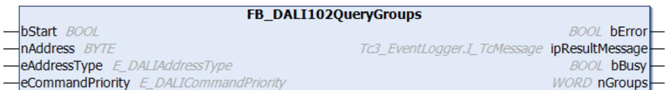
The function block reads the variable [gearGroups](#) [▶ 154] from the DALI control gear.
