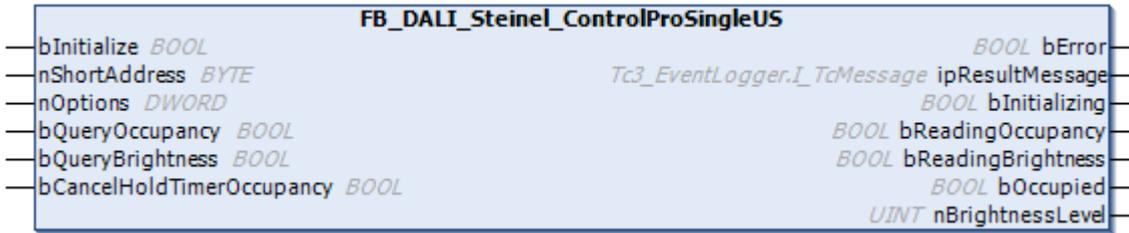
The function block represents the DALI ControlPro Single US DALI sensor from Steinel.
