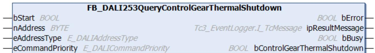
The function block indicates whether there is a thermal shutdown of the DALI control gear.
