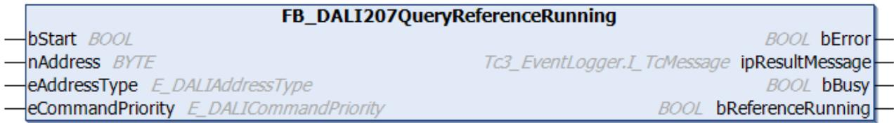
The function block queries whether a reference measurement of the system power is activated.
