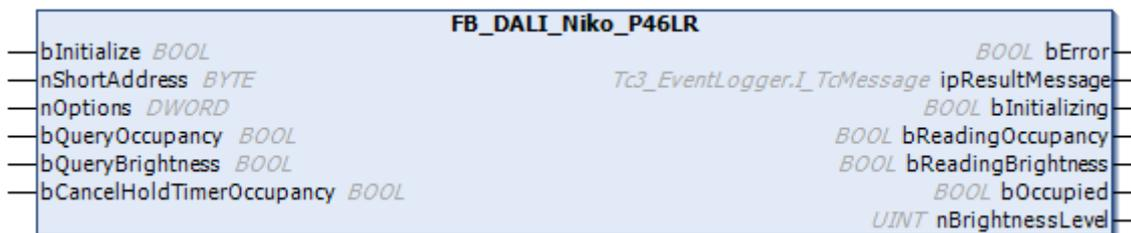
The function block represents the DALI sensors P46LR for surface mounting, P46LR for SnapFit flush mounting and P46LR for flush-mounting box from Niko.
