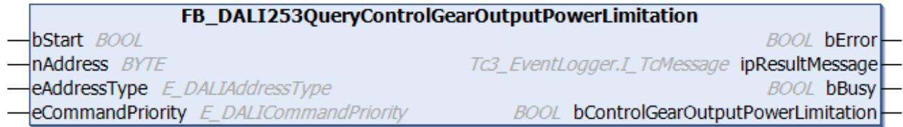
The function block indicates whether the limit value of the output power of the DALI control gear was exceeded.
