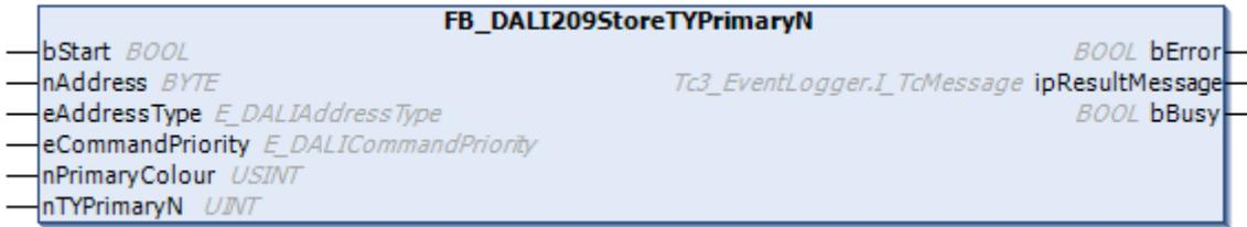
The function block stores the value `nTYPrimaryN` in the variable `tyPrimaryN` [▶ 419] of the DALI control gear.
