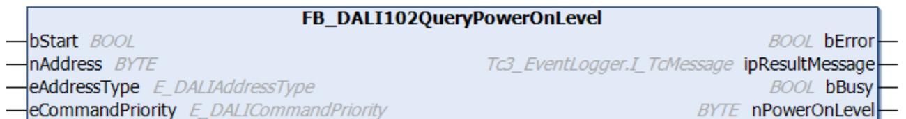
The function block reads the variable [powerOnLevel \[▶ 150\]](#) from the DALI control gear.
