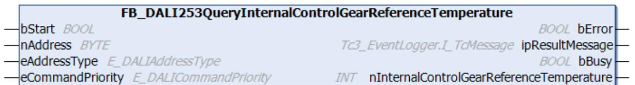
The function block outputs the internal reference temperature of the DALI control gear.
