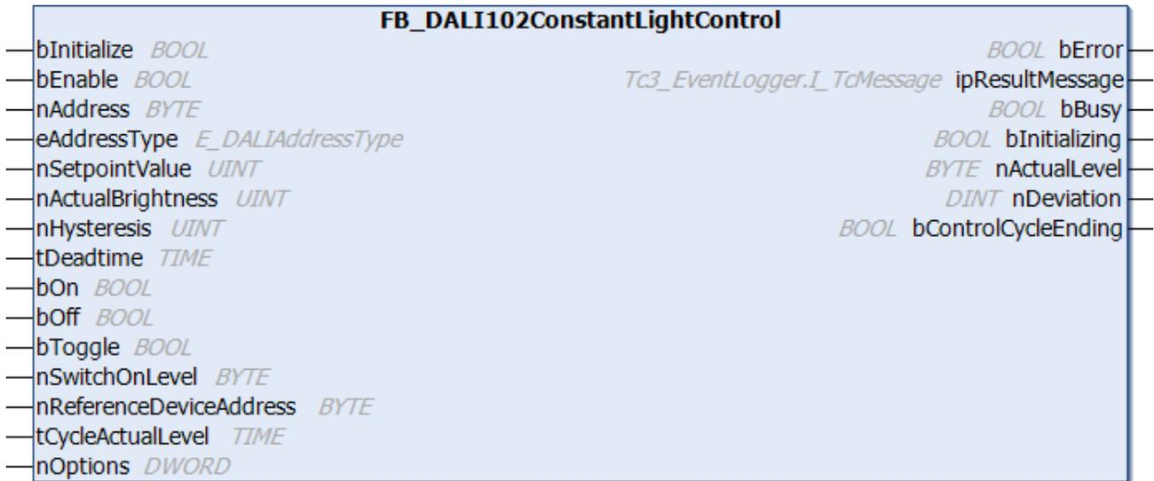
The FB\_DALI102ConstantLightControl function block provides the basic functions for implementing constant light regulation.
