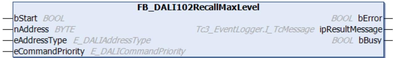
The output value of the DALI control gear is set to `maxLevel` [▶ 150].
