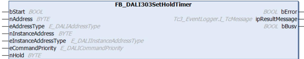
The function block stores the value of *nHold* in the variable *tHold* [▶ 560] of the DALI control device.
