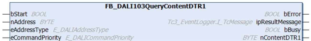
The function block reads the contents of [DTR1 \[▶ 229\]](#) (Data Transfer Register 1) from the DALI control device.
