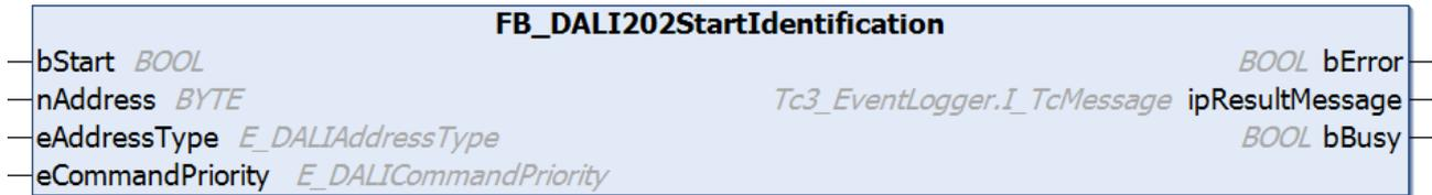
The function block starts or extends the identification routine of the DALI control gear.
