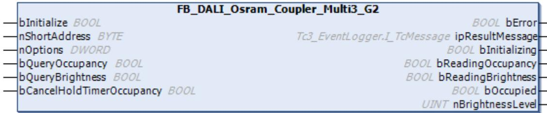
The function block represents the DALI COUPLER MULTI3 G2 DALI sensor from Osram.
