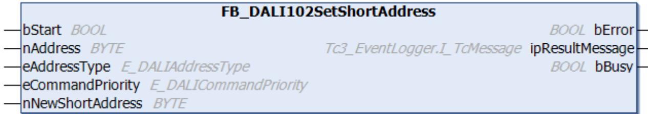
The function block stores the new short address *nNewShortAddress* in the shortAddress [▶ 153] variable of the DALI control gear.
