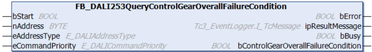
The function block outputs the status of `controlGearFailure` [▶ 153] at the DALI control gear.
