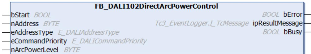
The function block switches the DALI control gear to the default output value *nArcPowerLevel*.
