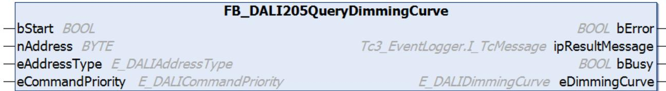
The function block reads the set dimming curve from the DALI control gear (see [dimmingCurve](#) [▶ 303]).
