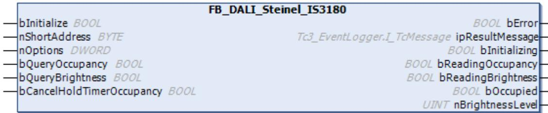
The function block represents the IS 3180 AP/UP DALI<sup>®</sup> sensor from Steinel.
