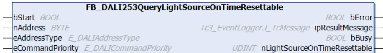
The function block reads the resettable operating hour counter of the light source. If the light source is switched on, the resettable operating hour counter is incremented by one every second. The resettable operating hours counter can be changed by the function block [FB\\_DALI253SetLightSourceOnTimeResettable](#) [▶ 505].
