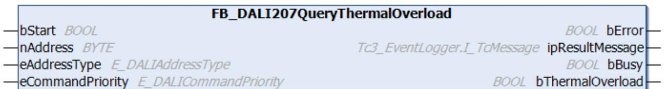
The function block queries whether there is a thermal overload with reduction of the output level.
