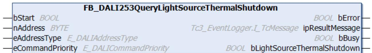
The function block indicates whether there is a thermal shutdown on the DALI control gear due to the light source.
