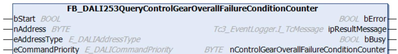
The function block reads the counter of the error events that have occurred in the DALI control gear.
