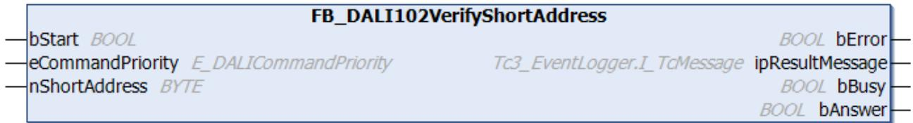
The function block checks whether the variable [shortAddress](#) [[▶ 153](#)] matches the value *nShortAddress* for all selected DALI control gears.
