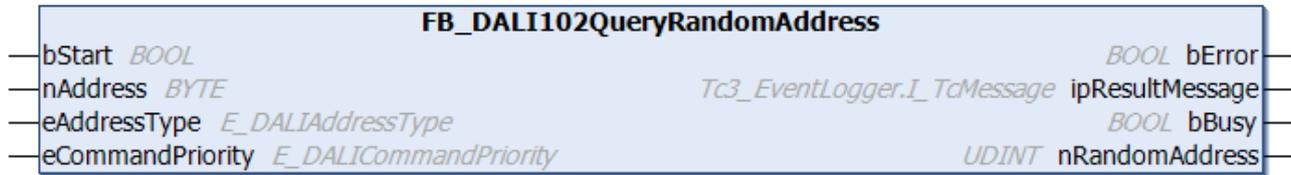
The function block reads the variable `randomAddress` [► 153] from the DALI control gear.
