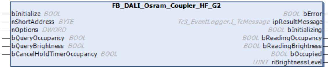
The function block represents the DALI COUPLER HF G2 DALI sensor from Osram.
