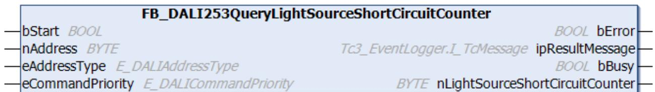
The function block reads the counter that counts the number of light source short-circuits.
