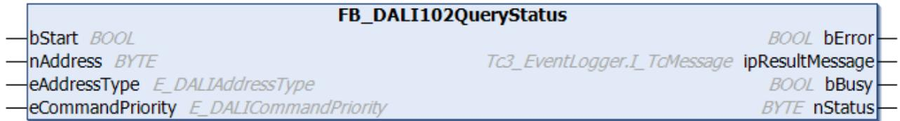
The function block reads the status of the DALI control gear.
