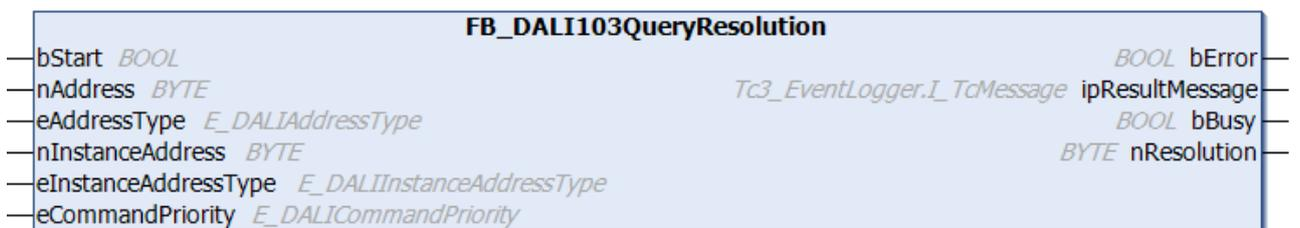
The function block reads the resolution of the input value for the selected instance from the DALI control device (see [resolution](#) [▶ 232]).
