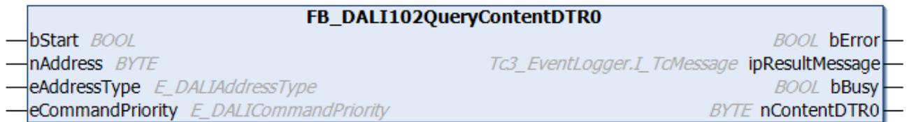
The function block reads the contents of [DTR0](#) [▶ 154] (Data Transfer Register 0) from the DALI control gear.
