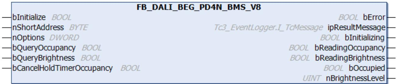
The function block represents the PD4N-BMS DALI-2 DALI sensor from B.E.G..
