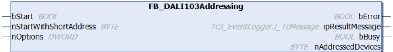
This function block addresses the DALI control devices at random. The user has no influence on which control device is assigned which short address. Short addresses are allocated in ascending order.
