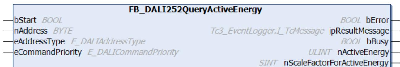
The function block reads the active energy from the DALI control gear.
