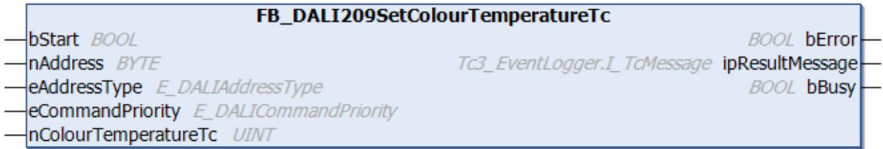
The function block saves the value *nColourTemperatureTc* in the variable *colourTemperatureTc* [▶ 419] of the DALI control gear and causes the set color temperature to be applied to the lamp by executing the ACTIVATE command.
