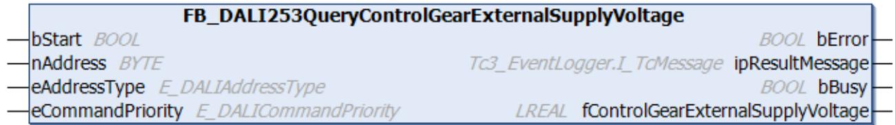
The function block reads the effective value of the external supply voltage from the DALI control gear.
