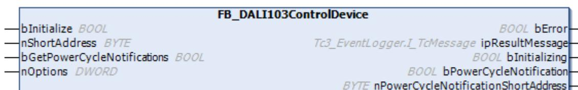
The function block is used for the configuration and operation of a DALI control device that supports Part 103 (control devices).
