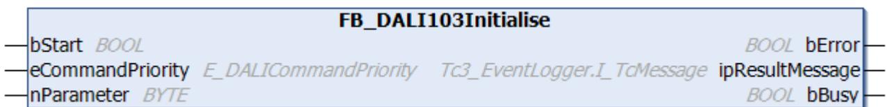
The function block prepares the addressing of the DALI control devices.
