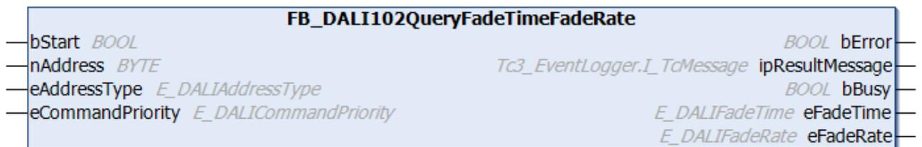
The function block reads the variables `fadeTime` [▶ 151] and `fadeRate` [▶ 150] from the DALI control gear.
