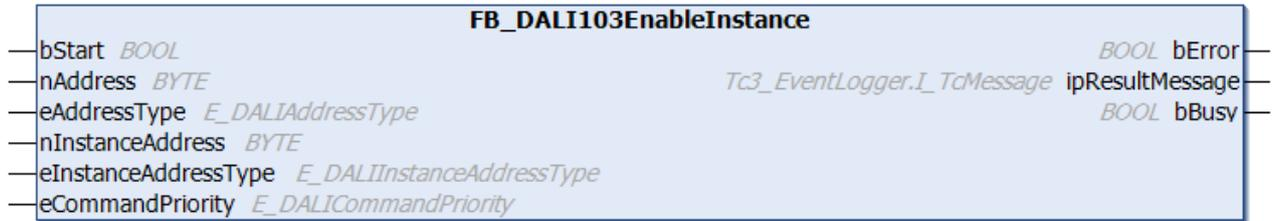
The function block enables the selected instance of the DALI control device (see [instanceActive](#) [▶ 232]).
