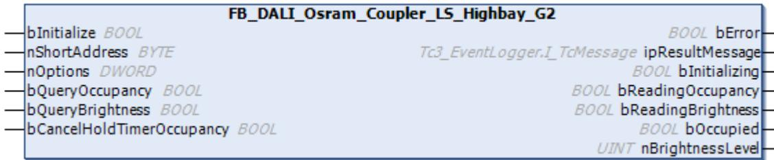
The function block represents the DALI COUPLER LS HIGHBAY G2 DALI sensor from Osram.
