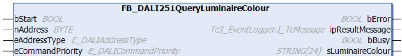
The function block reads the luminaire color from the DALI control gear.
