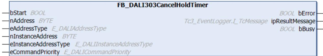
The function block ends the Hold Timer prematurely if the latter was implemented in the DALI control device.
