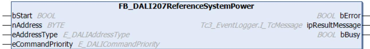
The DALI control gear measures and stores the performance level of the system, in order to detect load increase and decrease.
