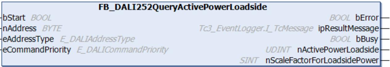
The function block reads the load-side active power from the DALI control gear.
