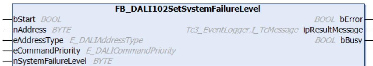
The function block stores the value *nSystemFailureLevel* in the variable [systemFailureLevel \[▶ 150\]](#) of the DALI control gear.
