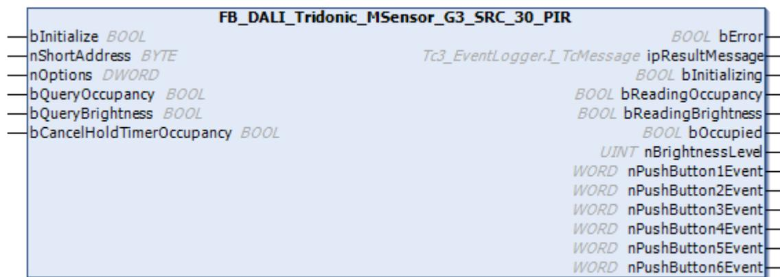
The function block represents the MSensor G3 SRC 30 PIR 5DPI DALI sensor from Tridonic.
