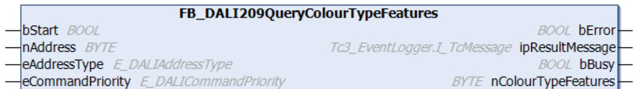
The function block reads the variable [colourTypeFeatures \[▶ 420\]](#) from the DALI control gear.
