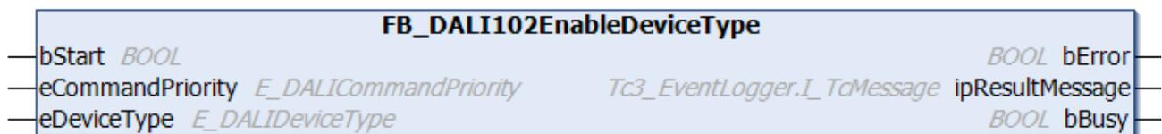
The function block must be called before an application extended command is called. This means that only the DALI control gears belonging to the corresponding device type respond.
