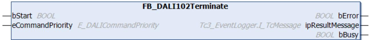
The function block terminates addressing for all DALI control gears. The selection of the DALI control gears to be addressed by the [FB\\_DALI102Initialise \[► 131\]](#) function block is also canceled.
