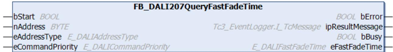
The function block reads the variable `fastFadeTime` [▶ 330] from the DALI control gear.
