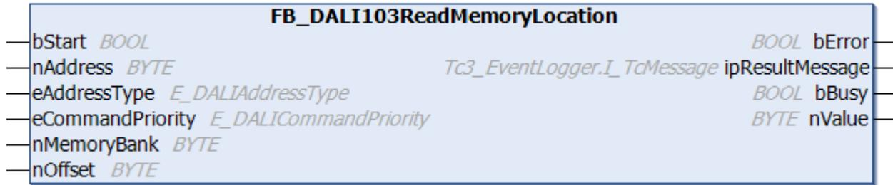
The value *nValue* is read from the memory bank of the DALI control device. The corresponding memory bank is specified by the input variable *nMemoryBank*, the address within the memory bank by the input variable *nOffset*.
