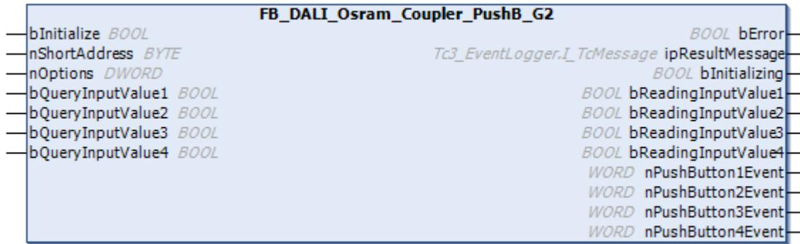
The function block represents the DALI COUPLER PushB G2 DALI push button interface from Osram.
