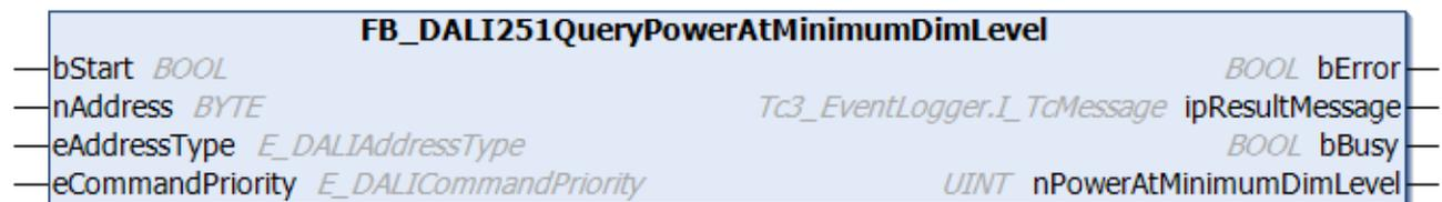
The function block reads the power consumption at the minimum dimming value of the DALI control gear.
