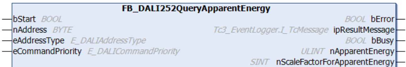
The function block reads the apparent energy from the DALI control gear.
