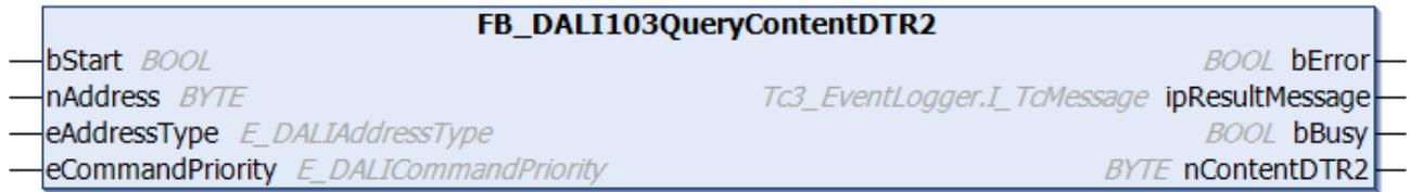
The function block reads the contents of DTR2 [[▶ 229](#)] (Data Transfer Register 2) from the DALI control device.
