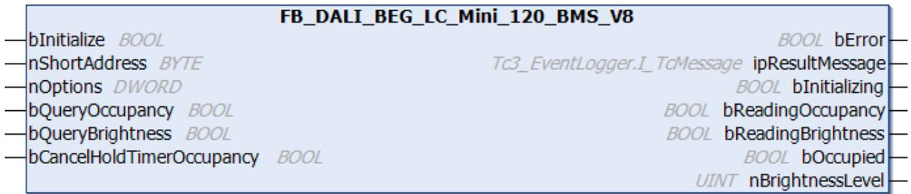
The function block represents the LC-Mini 120-BMS DALI-2 DALI sensor from B.E.G..
