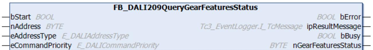
The function block reads the variable [gearFeatures/Status](#) [▶ 420] from the DALI control gear.
