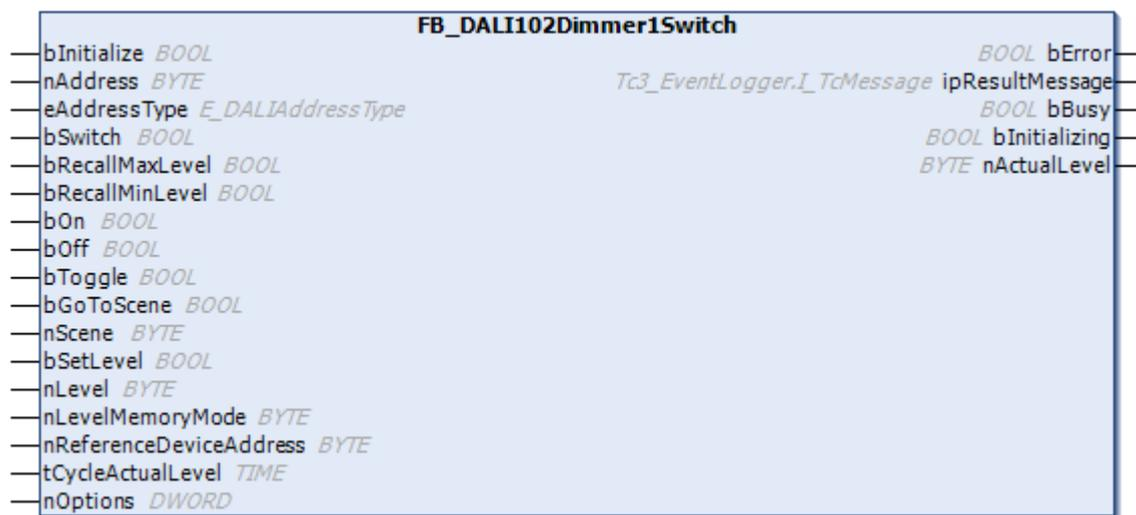
The function block FB\_DALI102Dimmer1Switch provides the main functions for implementing a push-dimmer.
