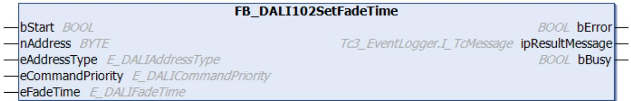
The function block sets the [fadeTime](#) [[▶ 151](#)] to the value *eFadeTime*.
