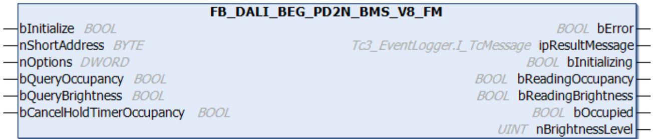
The function block represents the PD2N-BMS-V8-FM DALI-2 DALI sensor from B.E.G..
