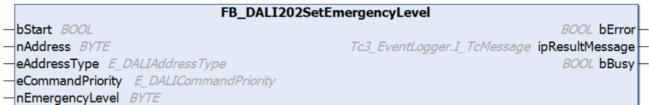
The function block stores the value *nEmergencyLevel* in the variable [emergencyLevel \[▶ 280\]](#) of the DALI control gear.
