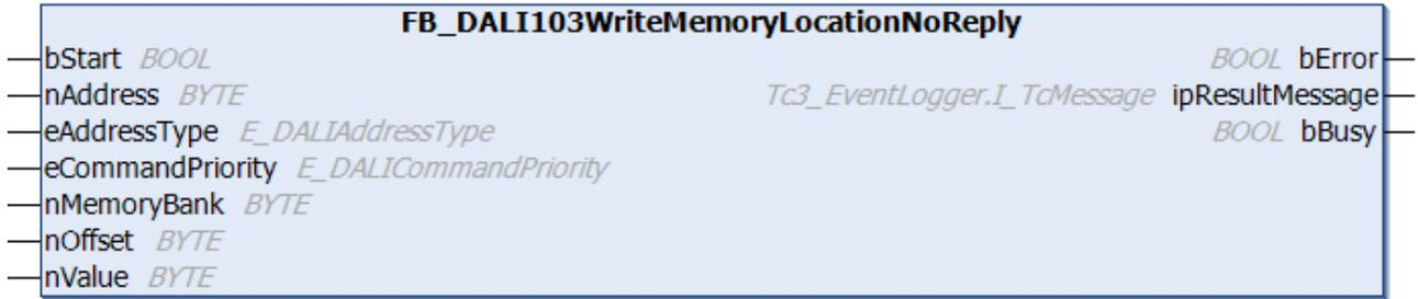
The value *nValue* is written in the memory bank of the DALI control device. The corresponding memory bank is specified by the input variable *nMemoryBank*, the address within the memory bank by the input variable *nOffset*.
