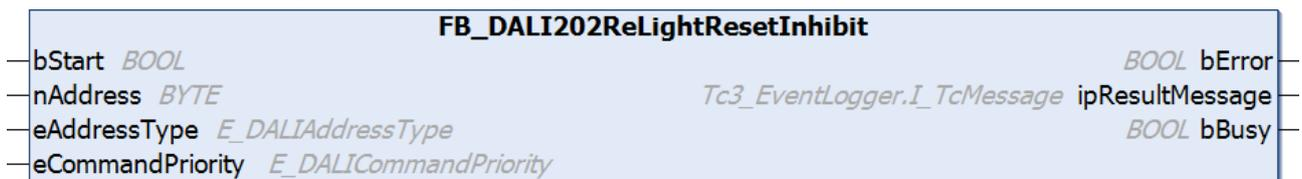
This function block is used to switch the DALI control gear back to emergency mode in the absence of mains voltage.
