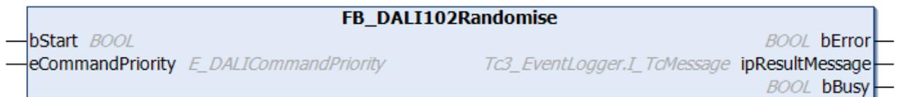
The function block generates a new random address for all selected DALI control gears and writes it to the [randomAddress \[▶ 153\]](#) variable.
