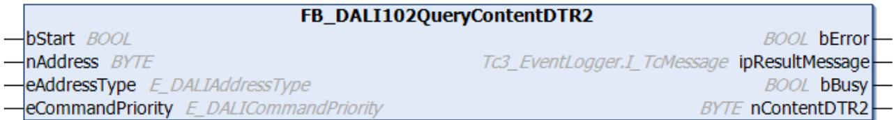
The function block reads the contents of [DTR2 \[► 154\]](#) (Data Transfer Register 2) from the DALI control gear.
