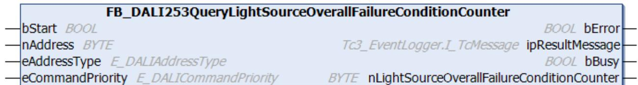
The function block reads the counter of the light source error events.
