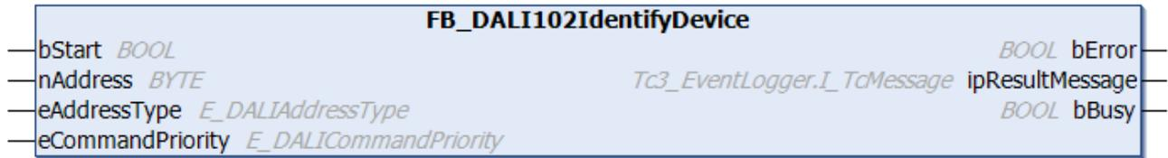
The function block starts the identification routine for the DALI control gear.
