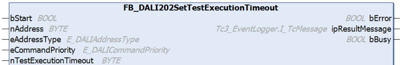
The function block stores the value *nTestExecutionTimeout* in the variable [testExecutionTimeout](#) [▶ 282] of the DALI control gear.
