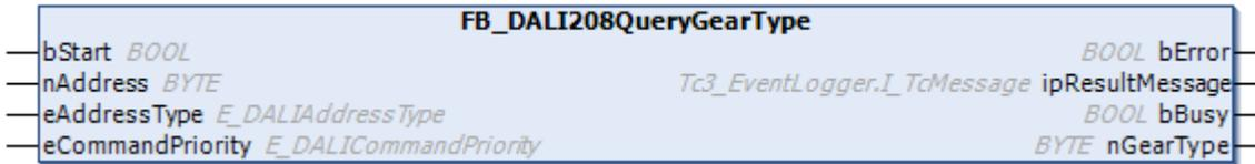
The function block reads the variable `gearType` [▶ 351] from the DALI control gear.
