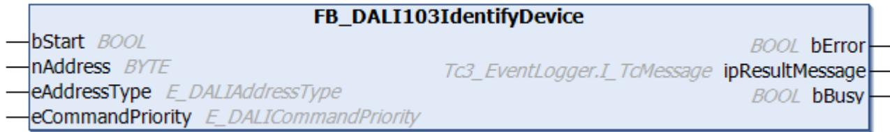
The function block starts the identification routine for a DALI control device.
