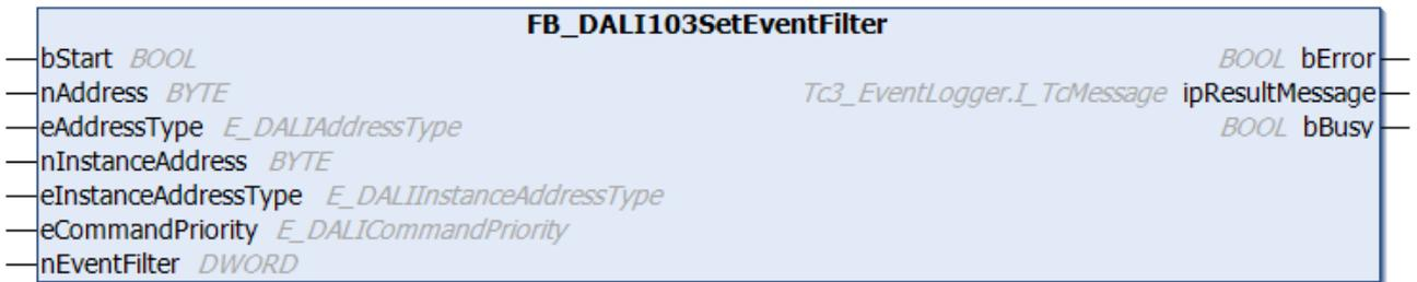
The function block sets the event filter (see [eventFilter](#) [[▶ 232](#)]) for the corresponding instance of the DALI control device.
