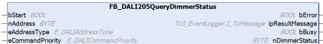
The function block reads the current operation mode from the DALI control gear (see [dimmerStatus](#) [[▶ 303](#)]).
