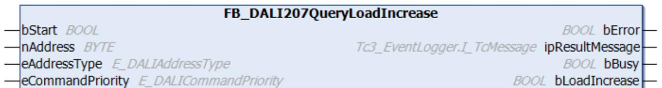
The function block queries whether a significant load increase (in comparison with the reference power of the system) has been detected.
