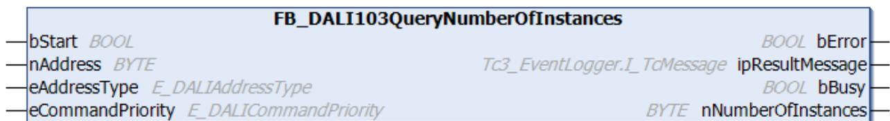
The function block reads the number of existing instances from the DALI control device (see [numberOfInstances \[▶ 230\]](#)).
