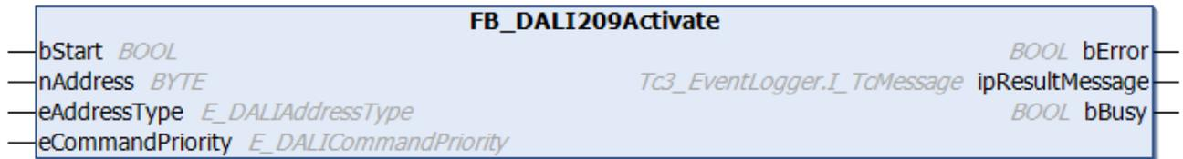
The function block causes the buffered values of the temporary registers to be transferred to the lamp. It ends a running cross-fade and starts a new cross-fade for the respective color/color temperature.
