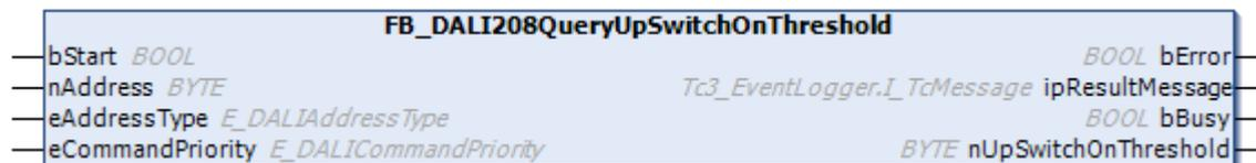
The function block reads the variable [upSwitchOnThreshold](#) [▶ 350] from the DALI control gear.
