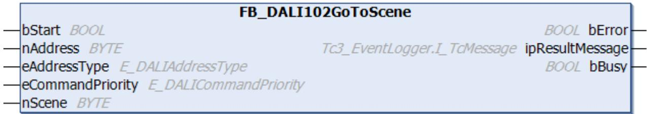
The output value of the DALI control gear is set to the value stored in *nScene*.
