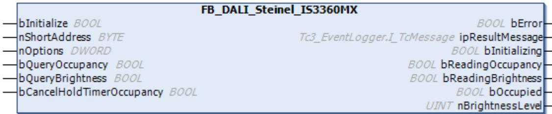
The function block represents the IS 3360 MX AP/UP DALI sensor from Steinel.
