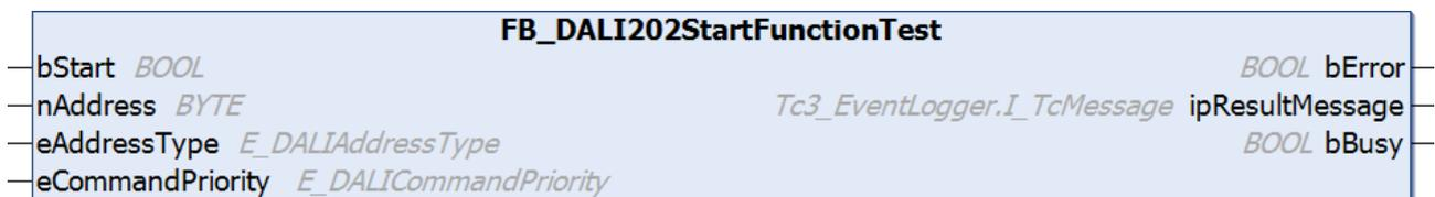
The function block starts a function test.
