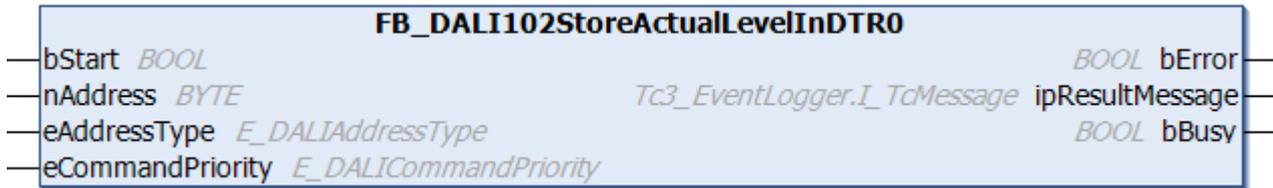
The function block writes the current output value of the DALI control gear to DTR0 [▶ 154].
