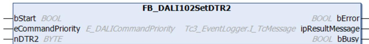
The function block writes to the [DTR2](#) [▶ 154] (Data Transfer Register 2) of all DALI control gears.
