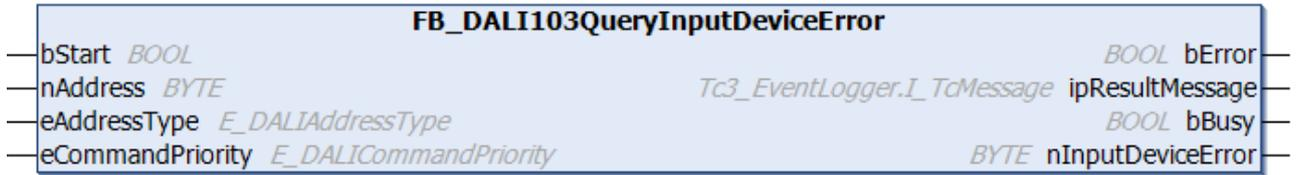
The function block reads more detailed error information from the DALI control device (see [inputDeviceError](#) [▶ 231]).
