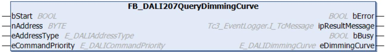
The function block reads the set dimming curve from the DALI control gear (see [dimmingCurve](#) [▶ 331]).
