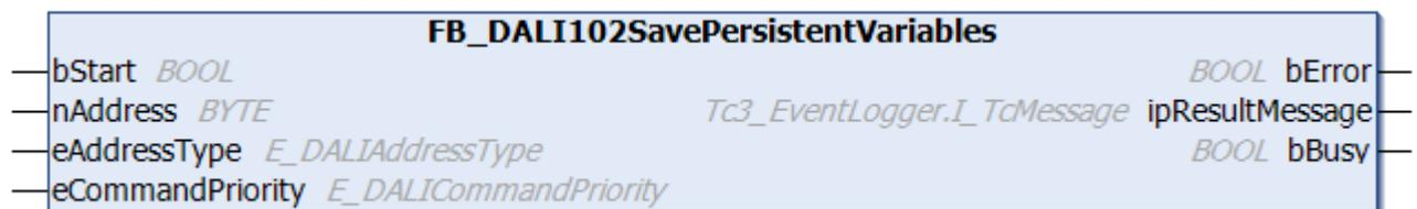
The function block immediately triggers the saving of variables in the persistent memory by the DALI command SAVE PRESISTENT VARIABLES.
