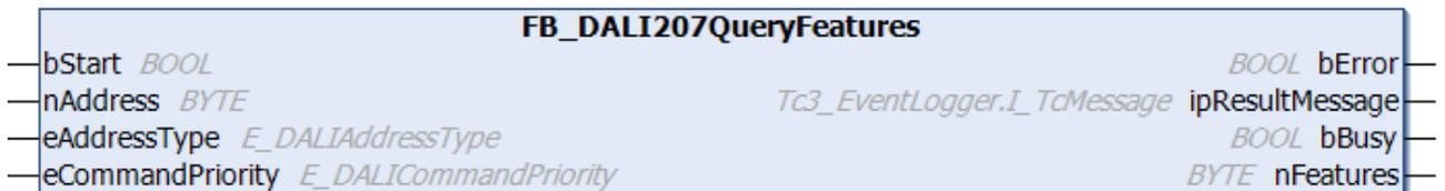
The function block reads the variable [features \[▶ 330\]](#) from the DALI control gear.
