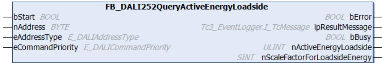
The function block reads the load-side active energy from the DALI control gear.
