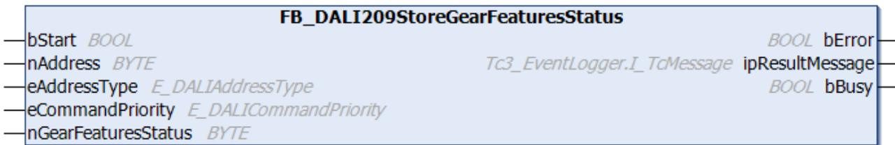
The function block saves the value *nGearFeaturesStatus* in the variable [gearFeatures/Status \[► 420\]](#) of the DALI control gear.
