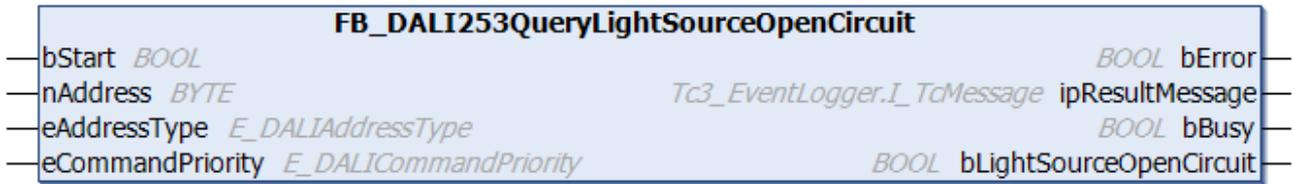
The function block indicates whether there is an open circuit to the light source.
