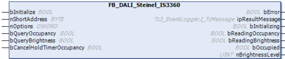
The function block represents the IS 3360 AP/UP DALI <sup>®</sup> sensor from Steinel.
