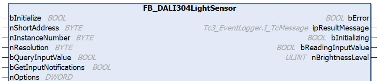
The function block is used for the configuration and operation of an instance of a DALI control device that supports Part 304 (light sensor).
