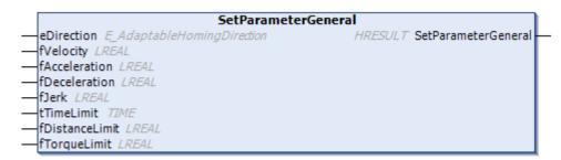
A set of travel parameters for the homing procedure is set.
