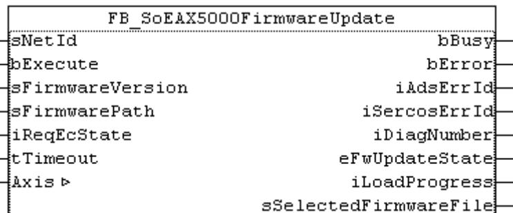
The functionblock FB\_SoEAX5000FirmwareUpdate can be used to check and update the firmware of the AX5000 to a requested version (revision and build) or to the newest build of the configured revision.
