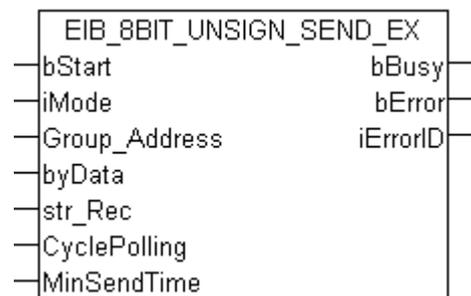
This function block sends an 8 Bit EIB value to the parameterized group address. As entry value there is an IEC61131--3 Byte-Variable. In dependence of the mode (*iMode*) the data can be sent manually, by polling or on change.
