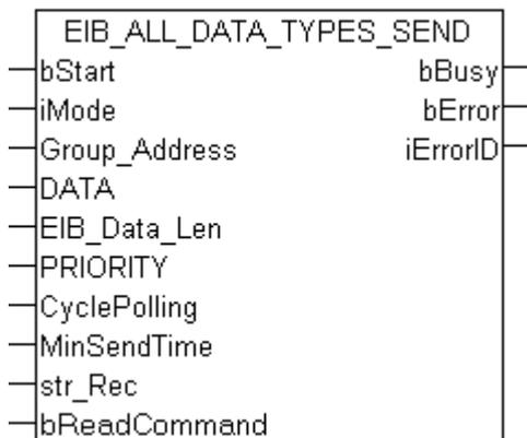
This function block sends a freely selectable EIB value to the set group address. An IEC61131-3 byte ARRAY variable is available as input value. The data are sent depending on the set mode.
