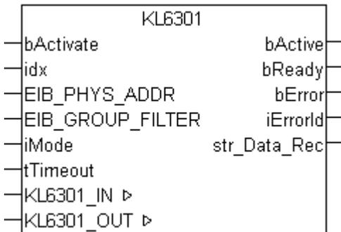
This function block deals with the KL6301 EIB Bus Terminal communication. It is used for configuring the KL6301 and for starting the data exchange with the EIB network.
