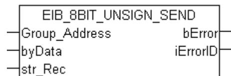
This function block sends a 8-bit EIB value to the set group address. An IEC61131-3 byte variable is available as input value. The data are only transferred if there is a change in the data value. If the value changes again within 1 second, new data are only sent to the EIB device after *minSendTime* has passed (see diagram). No new EIB telegram is sent if the value changes within the "min. send time" but falls back to the old, already sent value within the "min. send time".
