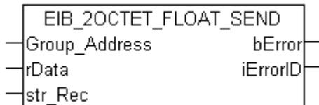
This function block sends a 2-byte float EIB value to the set group address. An IEC61131-3 real value is available as input value. The data are only transferred if there is a change. If the value changes again within 1 second, new data are only sent to the EIB device after another second has passed (see diagram). No new EIB telegram is sent if the value changes within the "min. send time" but falls back to the old, already sent value within the "min. send time".
