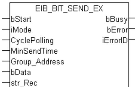
This function block sends an 1 Bit EIB value to the parameterized group address. In dependence of the mode (*iMode*) the data can be sent manually, by polling or on change.
