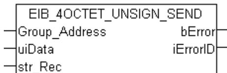
This function block sends a 4-byte unsign EIB value to the set group address. An IEC61131-3 UDINT value is available as input value. The data are only transferred if there is a change. If the value changes again within 1 second, new data are only sent to the EIB device after another second has passed (see diagram). No new EIB telegram is sent if the value changes within the "min. send time" but falls back to the old, already sent value within the "min. send time".
