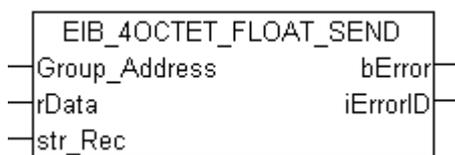
This function block sends a 4-byte float EIB value to the set group address. An IEC61131-3 REAL value is available as input value. The data are only transferred if there is a change. If the value changes again within 1 second, new data are only sent to the EIB device after another second has passed (see diagram). No new EIB telegram is sent if the value changes within the "min. send time" but falls back to the old, already sent value within the "min. send time".
