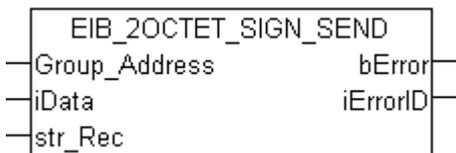
This function block sends a 2-byte sign EIB value to the set group address. An IEC61131-3 INT value is available as input value. The data are only transferred if there is a change. If the value changes again within 1 second, new data are only sent to the EIB device after another second has passed (see diagram). No new EIB telegram is sent if the value changes within the "min. send time" but falls back to the old, already sent value within the "min. send time".
