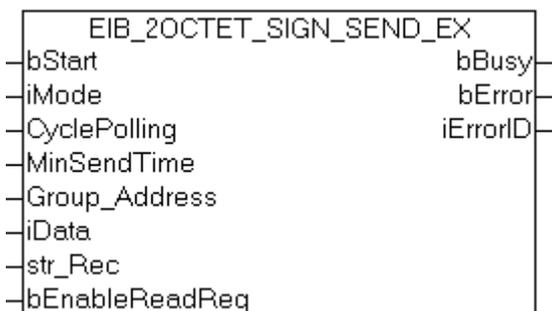
This function block sends a 2-byte sign EIB value to the set group address. An IEC61131-3 int value is available as input value. In dependence of the mode (*iMode*) the data can be sent manually, by polling or on change.
