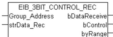
This function block receives 4 bits of EIB data on the set group address and converts them into an IEC61131-3 BOOL variable and a byte variable.
