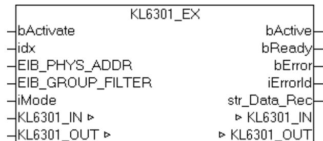
This function block deals with the KL6301 EIB Bus Terminal communication. It is used for configuring the KL6301 and for starting the data exchange with the EIB network.
