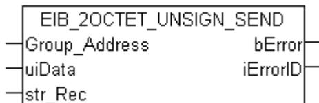
This function block sends a 2-byte unsign EIB value to the set group address. An IEC61131-3 UINT value is available as input value. The data are only transferred if there is a change. If the value changes again within 1 second, new data are only sent to the EIB device after another second has passed (see diagram). No new EIB telegram is sent if the value changes within the "min. send time" but falls back to the old, already sent value within the "min. send time".
