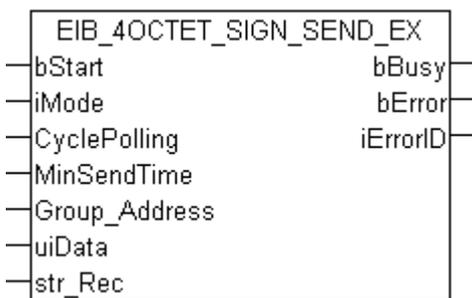
This function block sends a 4-byte sign EIB value to the set group address. An IEC61131-3 DINT value is available as input value. In dependence of the mode (*iMode*) the data can be sent manually, by polling or on change.
