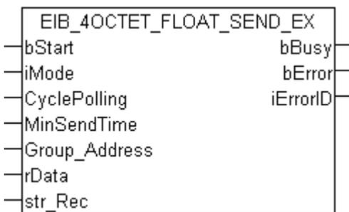
This function block sends a 4-byte float EIB value to the set group address. An IEC61131-3 real value is available as input value. In dependence of the mode (*iMode*) the data can be sent manually, by polling or on change.
