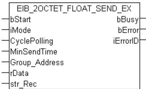
This function block sends a 2-byte float EIB value to the set group address. An IEC61131-3 real value is available as input value. In dependence of the mode (*iMode*) the data can be sent manually, by polling or on change.
