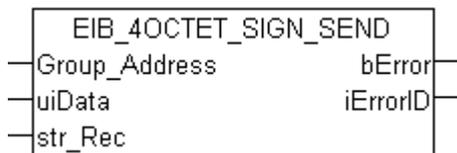
This function block sends a 4-byte sign EIB value to the set group address. An IEC61131-3 DINT value is available as input value. The data are only transferred if there is a change. If the value changes again within 1 second, new data are only sent to the EIB device after another second has passed (see diagram). No new EIB telegram is sent if the value changes within the "min. send time" but falls back to the old, already sent value within the "min. send time".
