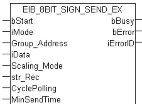
This function block sends an 8 Bit EIB value to the parameterized group address. As entry value there is an IEC61131-3 INT. By *Scaling\_Mode* the entry data value can be scaled. In dependence of the mode (*iMode*) the data can be sent manually, by polling or on change.
