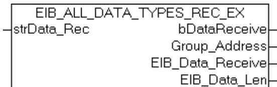
This function block receives variable EIB data sizes of all group addresses and outputs the raw data as a byte ARRAY.
