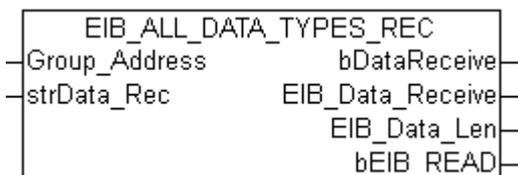
This function block receives variable EIB data sizes on the set group address and outputs the raw data as a byte ARRAY.
