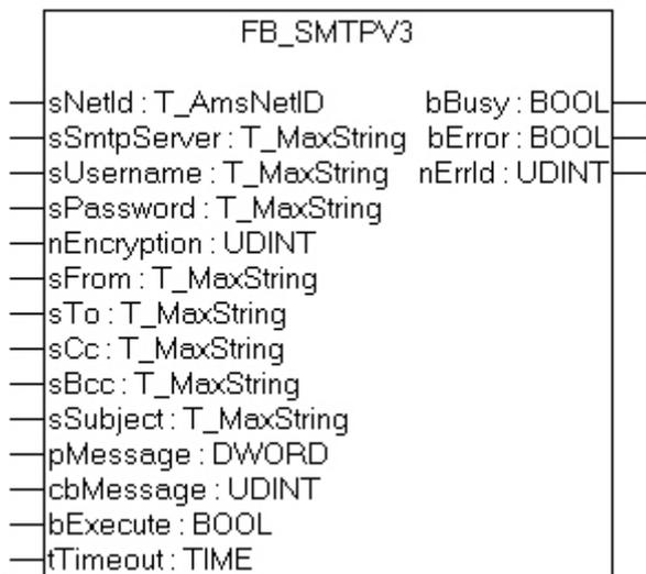
The block sends a byte stream to a remote ADS device via ADS. The TwinCAT ADS Smtplib service must be running on the remote ADS device, so that the byte stream can be received and processed into an e-mail. Once the byte stream has been processed the e-mail is sent.
