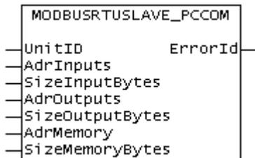
The function block *ModbusRTUslave\_PcCom* implements a Modbus slave that communicates via a serial PC interface (COM port). The block is passive until it receives telegrams from a connected Modbus master.
