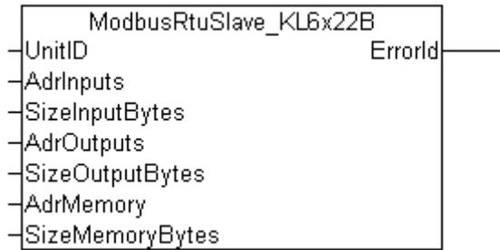
The function block *ModbusRtuSlave\_KL6x22B* implements a Modbus slave that communicates via a serial Bus Terminal KL6031 or KL6041. The block is passive until it receives telegrams from a connected Modbus master.
