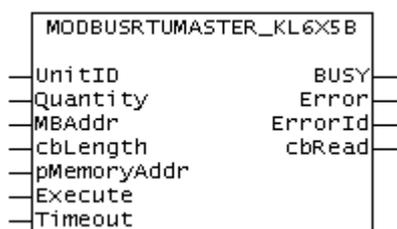
The function block *ModbusRtuMaster\_KL6x5B* implements a Modbus master that communicates via a serial Bus Terminal KL6001, KL6011 or KL6021. The block is not called in its basic form, but individual actions of that block are used within a PLC program. Each Modbus function is implemented as an action.
