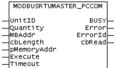
The function block *ModbusRtuMaster\_PcCom* implements a Modbus master that communicates via a serial PC interface (COM port). The block is not called in its basic form, but individual actions of that block are used within a PLC program. Each Modbus function is implemented as an action.
