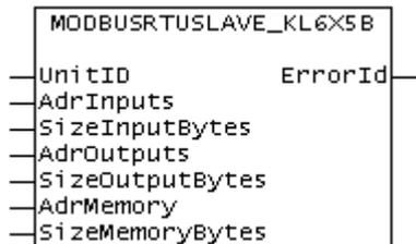
The function block *ModbusRtuSlave\_KL6x5B* implements a Modbus slave that communicates via a serial Bus Terminal KL6001, KL6011 or KL6021. The block is passive until it receives telegrams from a connected Modbus master.
