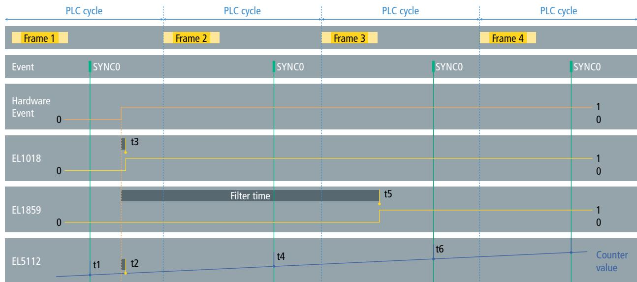
The illustration above shows the chronology of various events in relation to a hardware event that triggers latching. The statuses of the terminals and relevant bus events are displayed, as are the EtherCAT frames affected by jitter and the corresponding filter time (which is not necessarily proportional to the real filter times demonstrated by the terminals). The current position value is shown in blue.
