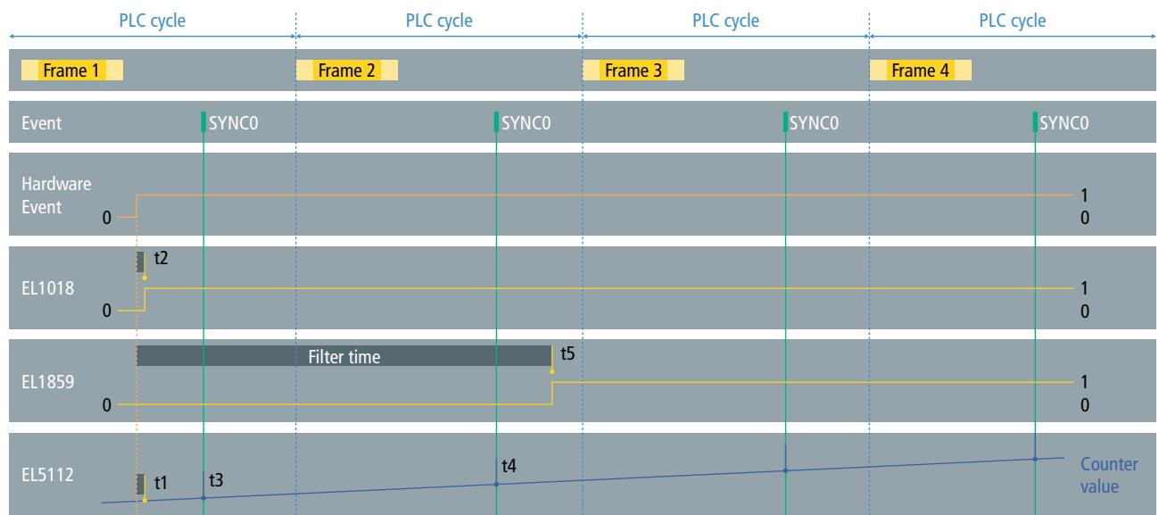
In this case, the latch position (t3) determined with the EL1018 in combination with the PLC is higher than the position determined by the EL5112 using the latch inputs (see t1). Although the EL1018 input is also valid in the first cycle (t2), as with the previous example, and is transmitted to the PLC with the second frame, the current position that is transmitted by the EL5112 is still determined at the SYNC0 event that now takes place after the hardware event.
