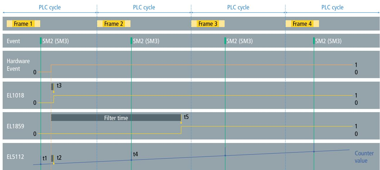
This means that the position value latched by the EL5112 (at point in time t2) is higher than the position determined by the PLC using the EL1018 (see t1). This applies vice versa to the input with a higher filter time (EL1859), and the position value that is determined by the PLC using the EL1859 (t4) is higher than the value latched by the EL5112.
